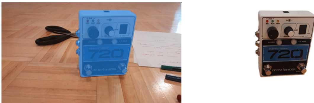
Figure 25: Image with object of interest segmented out.
