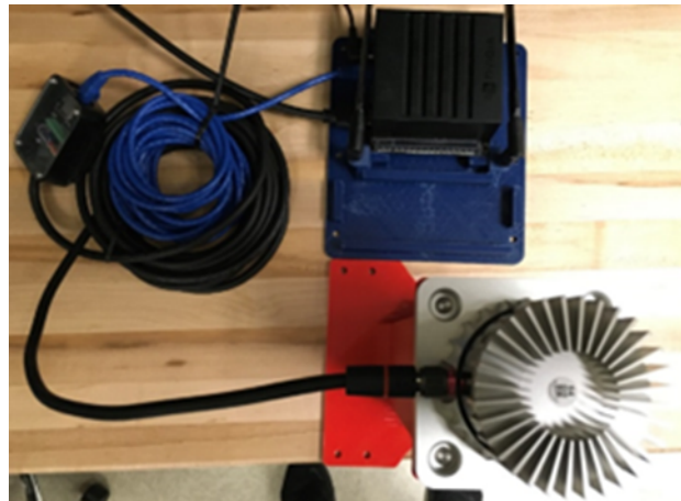
Figure 35: LiDAR unit with power supply and connection to the GPU.
