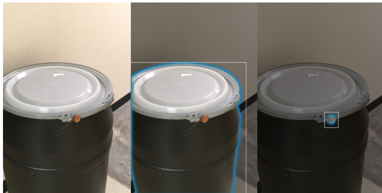
Figure 21: SAM segmentation from bounding boxes for drums and seals.
