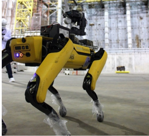
Figure 12: Spot, with a radiation detection payload, deployed at Chernobyl. Image from [15].
