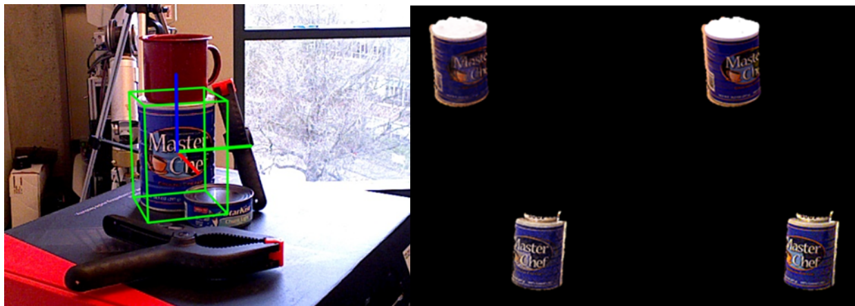
Figure 30: FoundationPose pose estimation from NERF for objects with unknown models.
