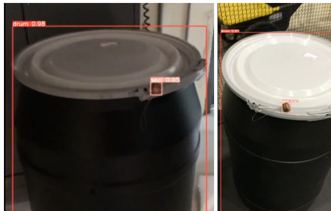
Figure 18: Test results for object detection of 55-gallon drums and metal cup seals, with confidence level displayed.
