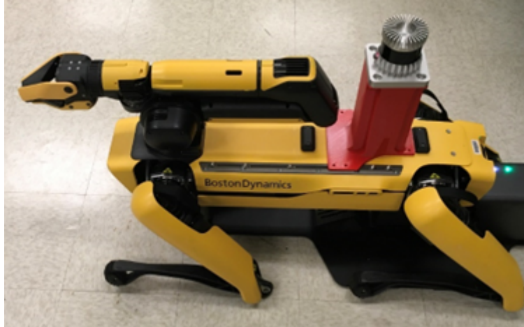
Figure 36: LiDAR mounted to Spot (GPU not shown but is typically mounted towards the back of Spot).
