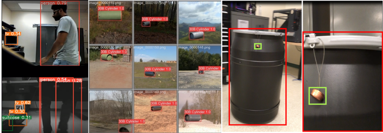
Figure 17: Progression of object detection training. (Left) COCO dataset for common objects, (Center) Limbo dataset for UF 6 and other cylinders, (Right) 55-gallon drums and metal cup seals at the AutonomyNM testbed.
