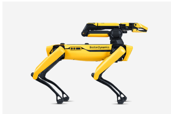
Figure 11: Boston Dynamics Spot robot with manipulator arm [14].
