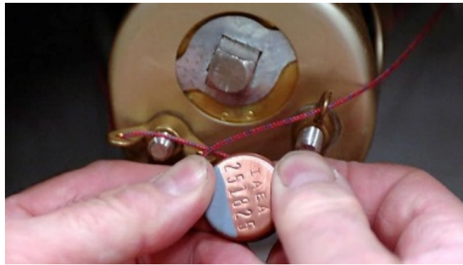
Figure 2: Metal cup seal. Image from [7].
