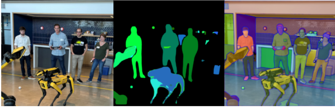
Figure 20: Pretrained segmentation results. Mask-RCNN in the middle. Segment Anything Model on the right.
