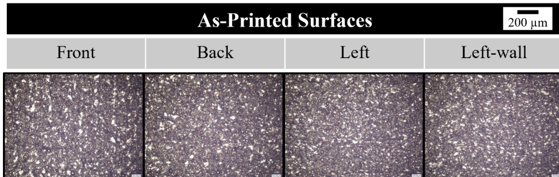
Figure 22. Optical images of as-printed surfaces for each surface orientation.
