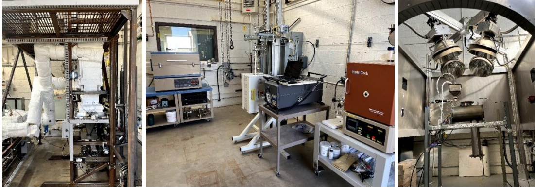
Figure 14. From left to right: test cell one (heat exchanger test stand), two (high temperature furnaces), and three (solar simulator) in the electric-heating test facility.
