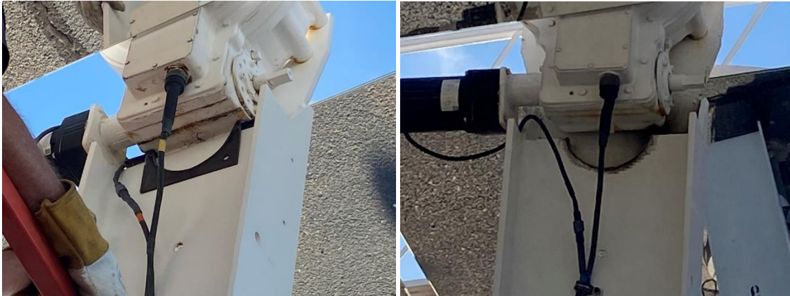
Figure 2. Elevation drive oil port access modifications to a heliostat shown before (left) and after (right) plasma cutting.
