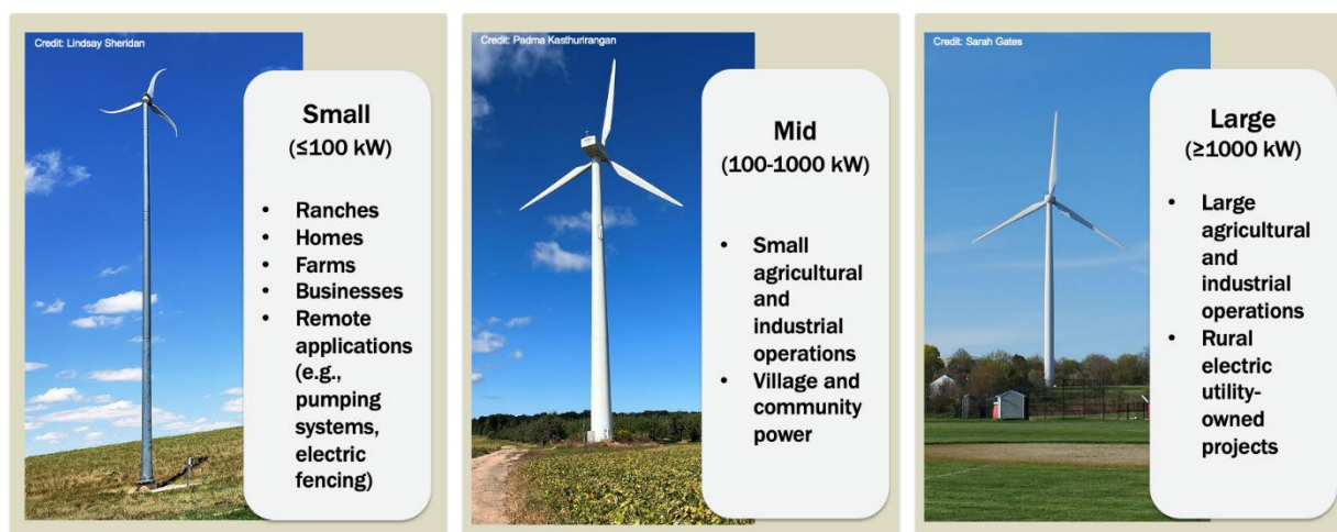
Figure 2. Categorical sizing of wind turbines and possible applications.
