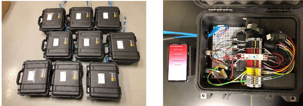
Figure 12 - Multiple HEM data acquisition system: In Pelican case (left) and components (right)
