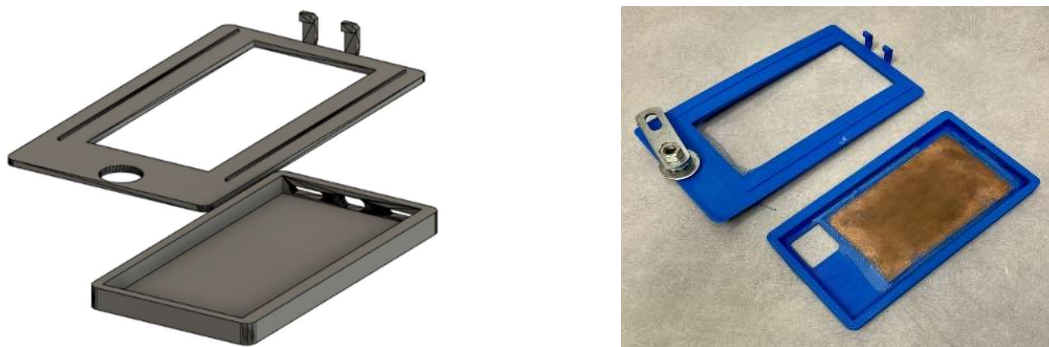
Figure 14 - Version 1 Case 3D Design (left) and Version 1 Case Printed and Assembled (right)
