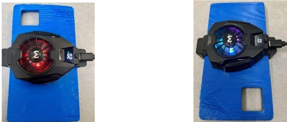
Figure 16 - Version 1 case temperature at beginning (left - 20°C ) and after 5 min (right - 10°C)
