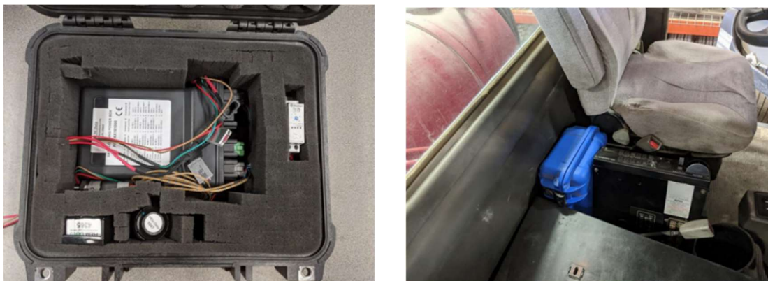
Figure 11 - HEM data acquisition system in Pelican case (left) and mounted in truck (right)
