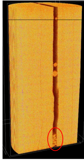
Fig. 8. 3D \mu -CT reconstruction, pre-MICP. Proppant accumulated at the bottom of the core during analysis (circled), though other particles are still firmly pressed between both sides of the fracture in other locations.
