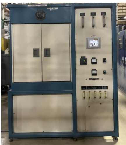
Figure 23. CM Hydrogen Atmosphere Batch Furnace
