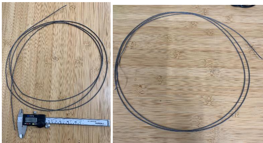
Figure 15. Images of composite 14YWT filaments that could be spooled.
