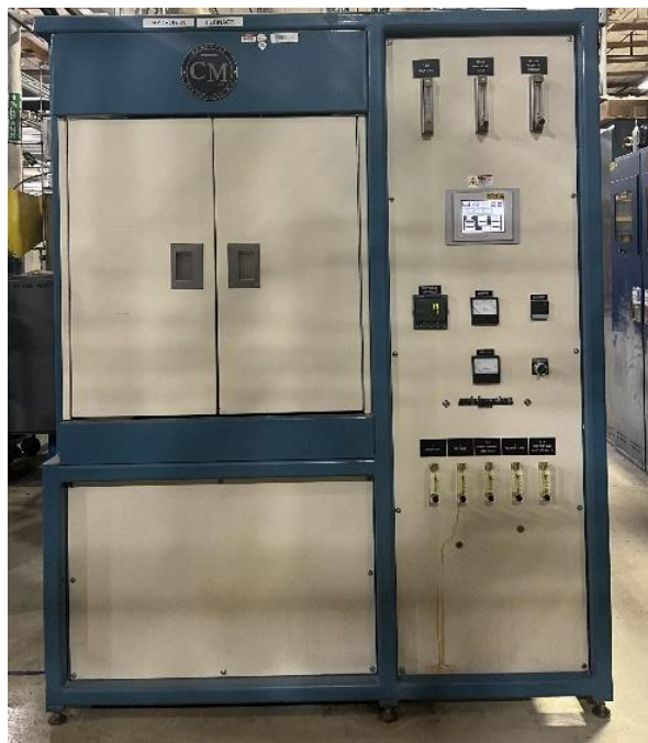
Figure 37. CM Hydrogen atmosphere batch furnace.
