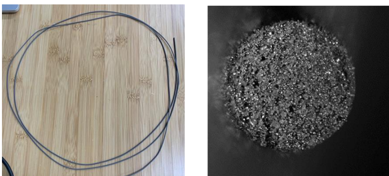
Figure 20. Filament loading 65% by volume fabricated from 14YWT 325 mesh spherical powder.
