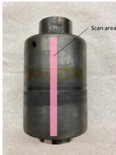
Figure 12. Diagram of surface scans taken on sleeve specimens.
