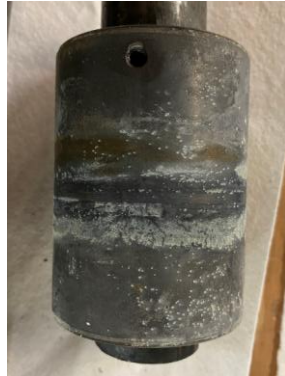
Figure 14. Shaft sleeves after removal from the inner column structure. There appears to be some corrosion outside of the contact areas and contact areas appear to be relatively clean.
