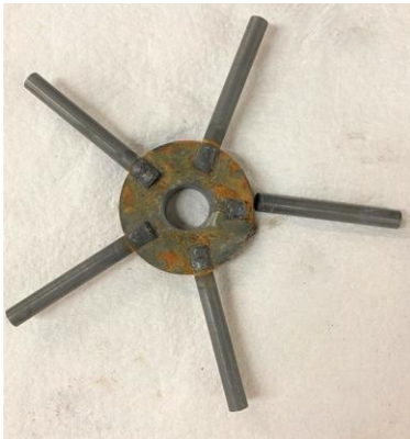
Figure 7. Pin specimen hub after removal from shaft. Pin samples are solid NiWC3B material
