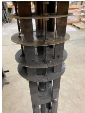
Figure 6. thermal isolation zones after salt test.
