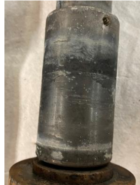
Figure 14. Shaft sleeves after removal from the inner column structure. There appears to be some corrosion outside of the contact areas and contact areas appear to be relatively clean.
