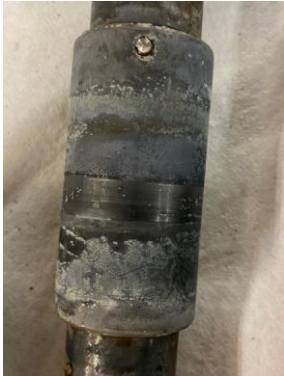
Figure 14. Shaft sleeves after removal from the inner column structure. There appears to be some corrosion outside of the contact areas and contact areas appear to be relatively clean.
