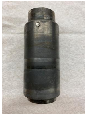
Figure 8. Upper shaft sleeve ( solid-NiWC3B-coated SS316 material ) after molten salt test.
