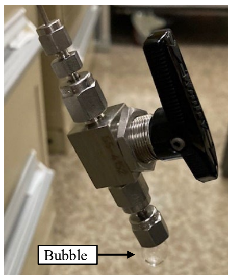
Figure 2-3. Water bubble forming at the sampling line outlet (bottom of photo, indicated by arrow) during 220°C drying process.
