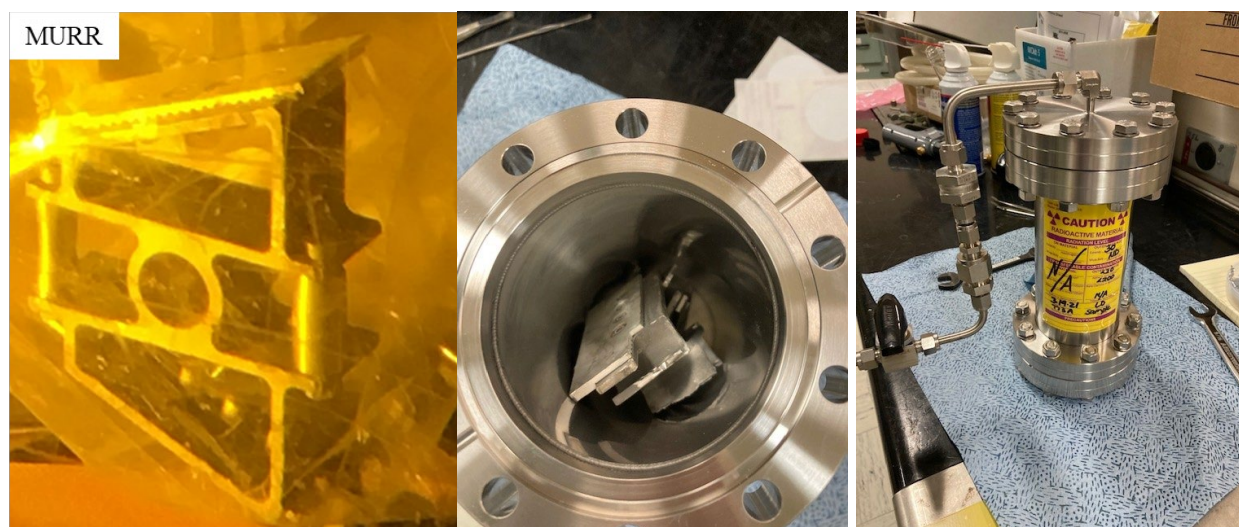
Figure 2-2. (Left) MURR cropping in shielded cells prior to characterization, (center) MURR cropping pieces loaded into the mini-canister, and (right) sealed MURR mini-canister with contamination filter.
