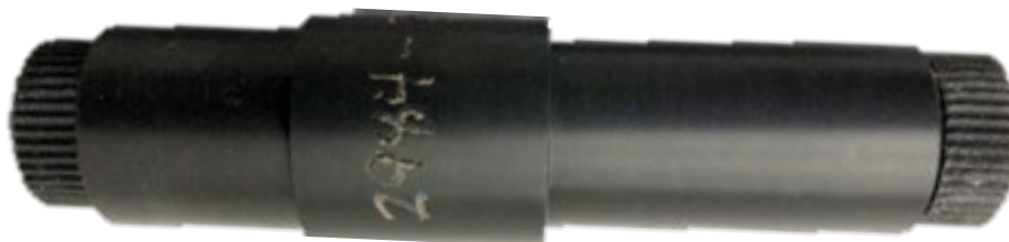
Figure 2-7. Photograph of a VLSJ Ag/AgCl reference electrode type that is currently used in Hanford DSTs (manufactured by Van London Co.). 21
