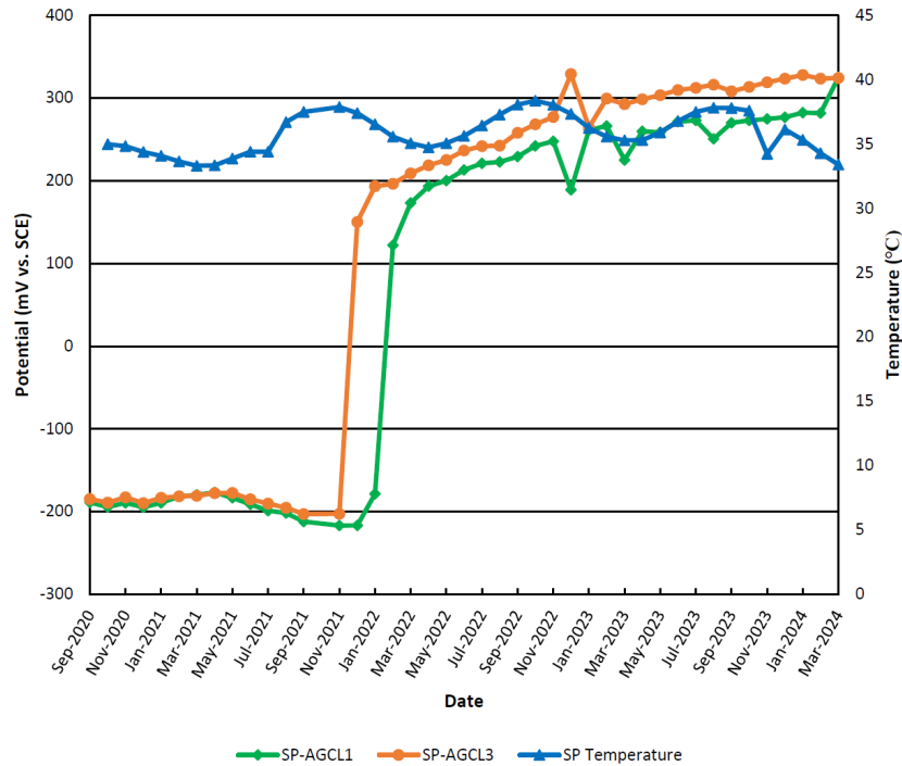
Figure 2-11. Corrosion Potential data collected from RCMP installed in Tank AP-102 from September 2020 to March 2024 17 .
