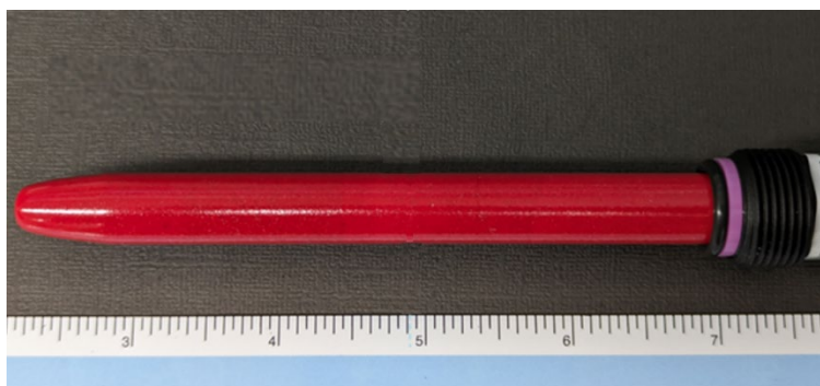
Figure 4-7. Photograph of a commercially available Reflex Ag/AgCl reference electrode.
