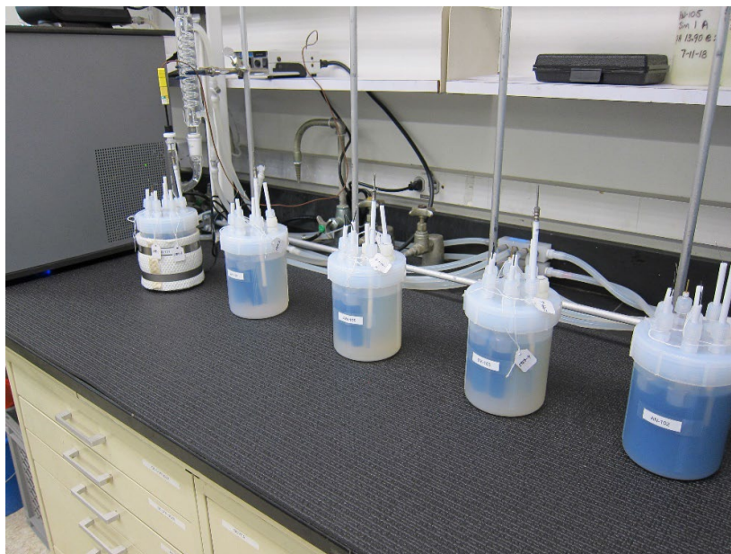
Figure 2-14. Photograph of a DNV test setup for long-term reference electrode study in various DST waste simulants 22 .
