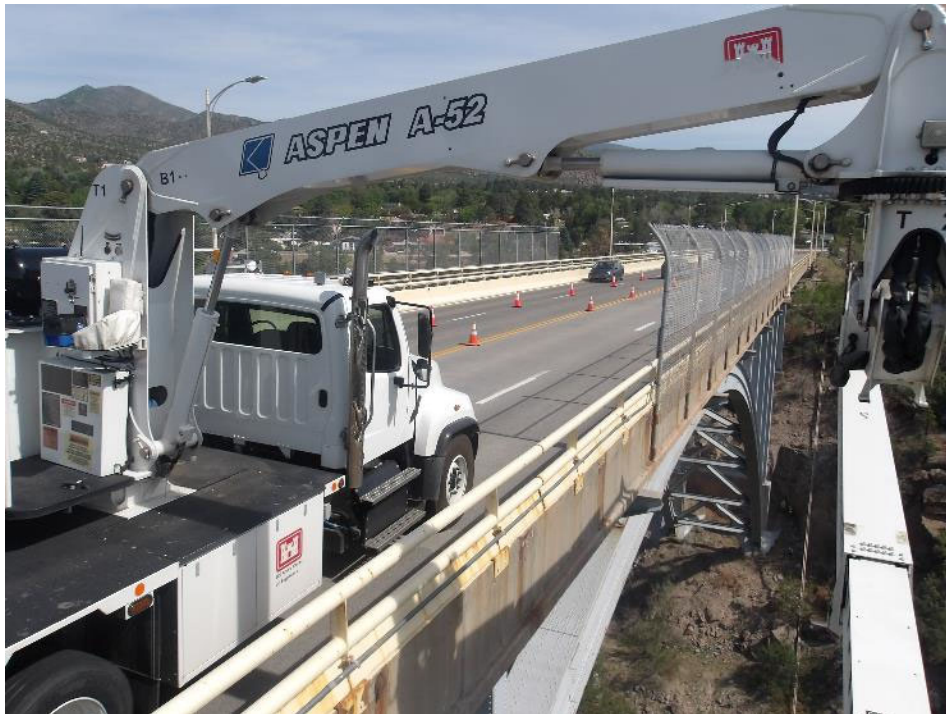
General Photo 6 – Use of under-bridge vehicle for inspection.
