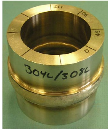
HAZ Cracking After Long-Term Exposure of Test Reservoir
