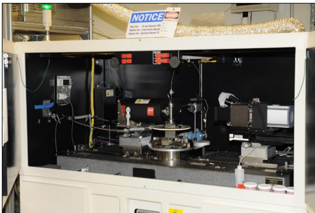
Figure 8: Zeiss Xradia MicroXCT-400 Micro-CT scanner used for high-resolution CT imaging at NETL.
