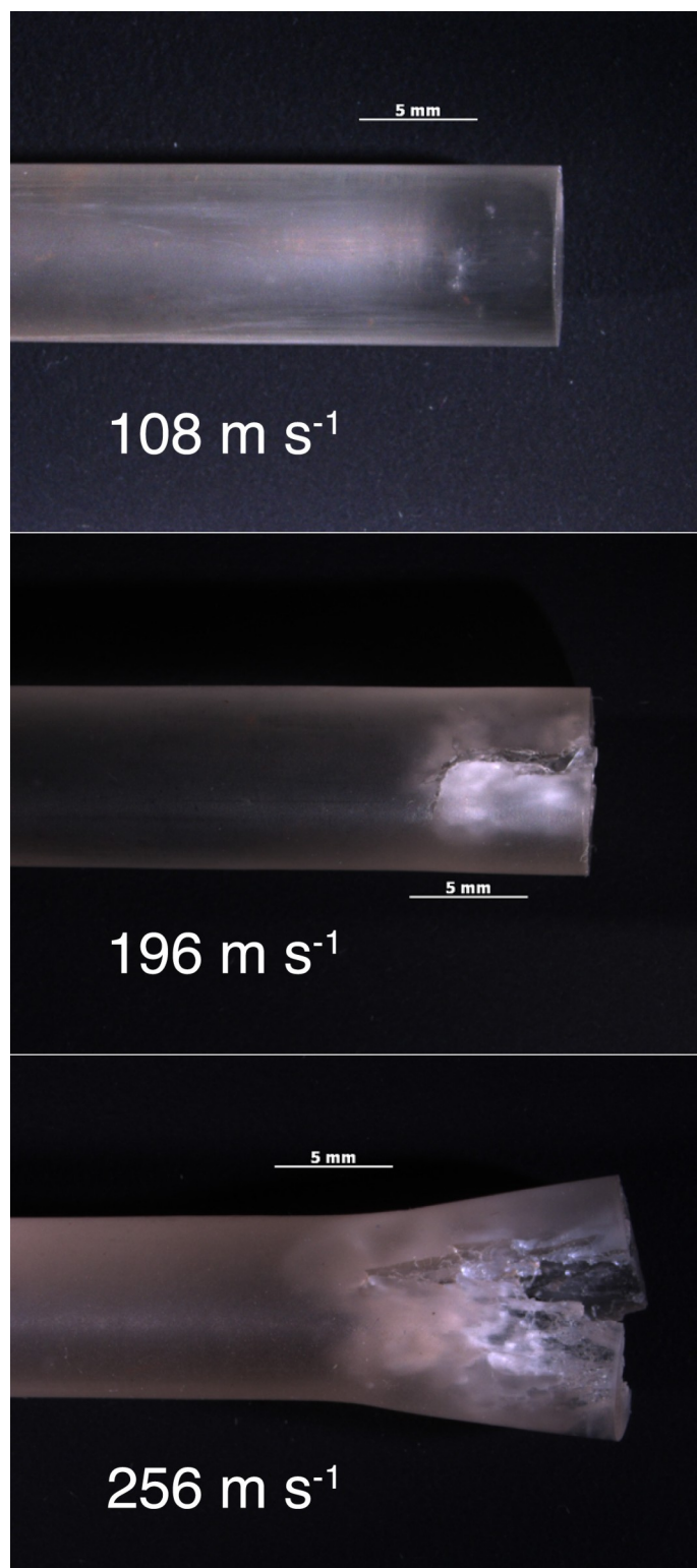
Figure 66. The room temperature (22°C) response of Kel-F 800 as a function of impact velocity.
