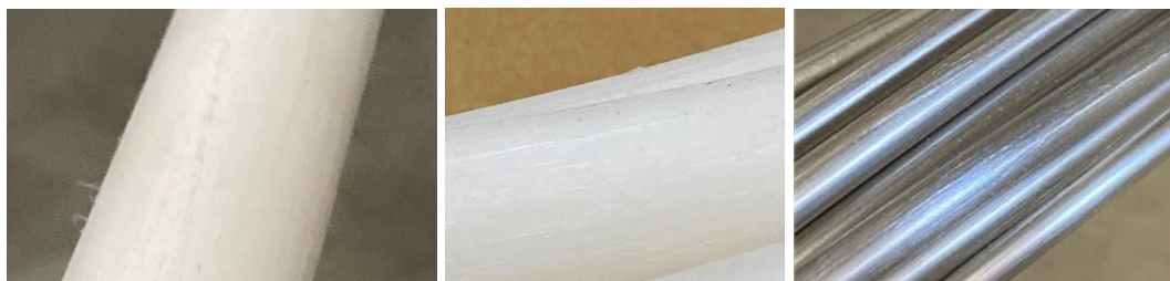
Figure 6. Surfaces roughened by sanding of the conveyance pipe, tremie pipe, and stainless-steel tubing.
