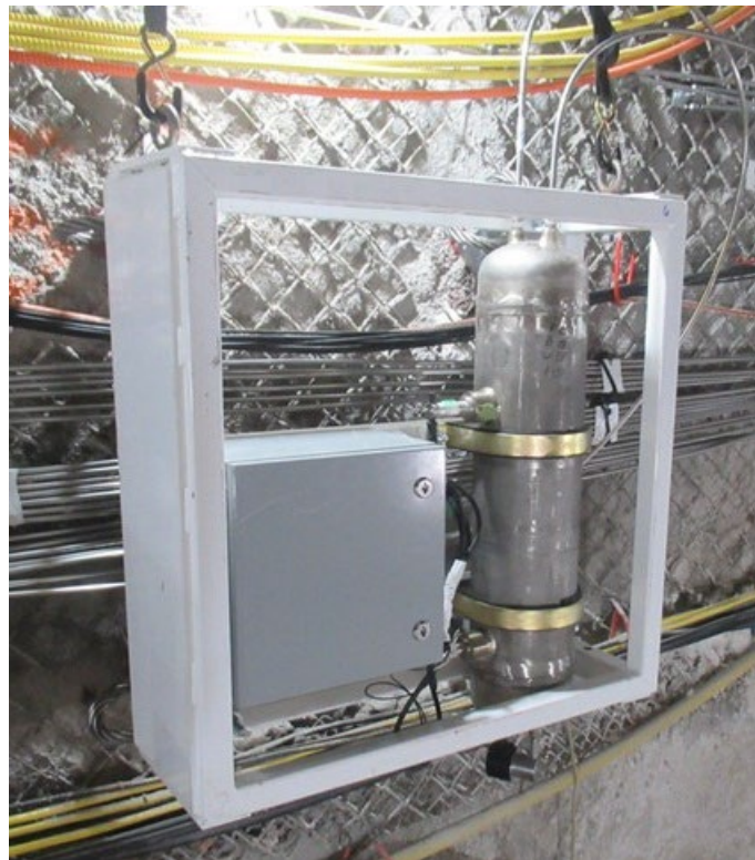
Figure C7. Water trap installed in tunnel.
