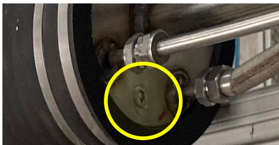
Figure H2. Packer air fill port on downhole side of packer (plugged).
