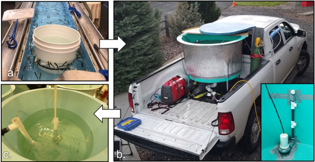
Fig. 1 Photographs of the a collection trough at McNary dam with lightly anesthetized American shad and a bucket of saltwater, b the transport tank in the bed of a pickup truck, and inside of the transport tank showing the water pump
