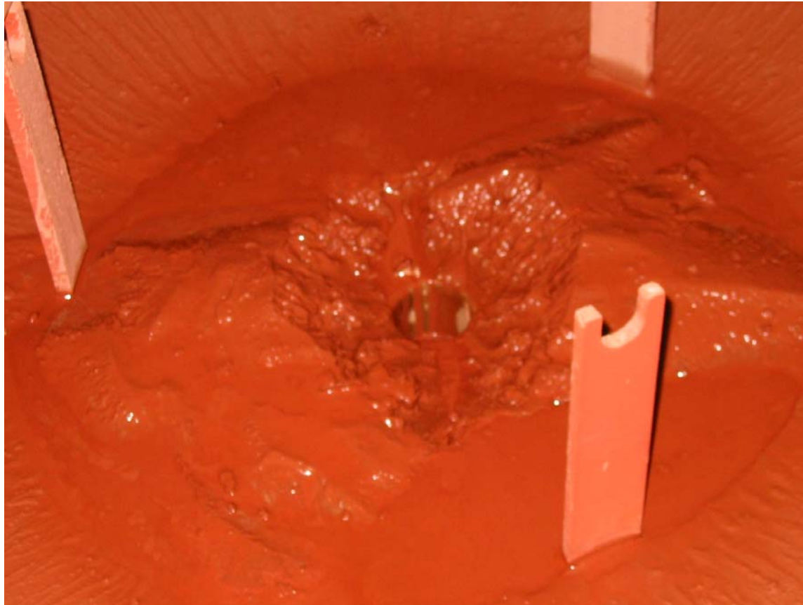
Figure 5.30. SBS bowl before cleaning at the end of the test.
