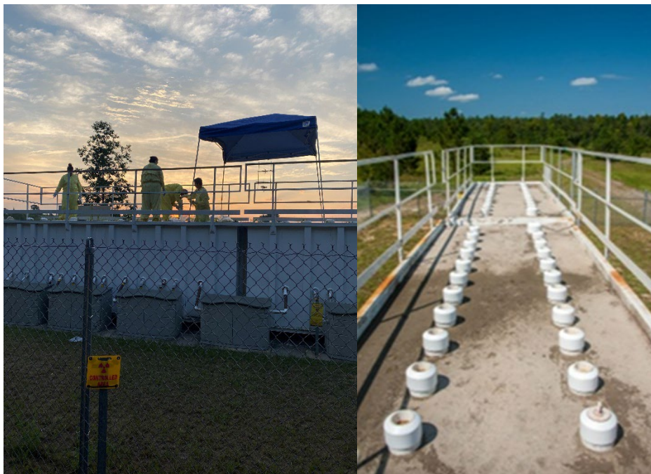
Figure 7. (Left) Soil cores being installed by SRNL operations and Radcon (Right) Cores installed on top of facility.
