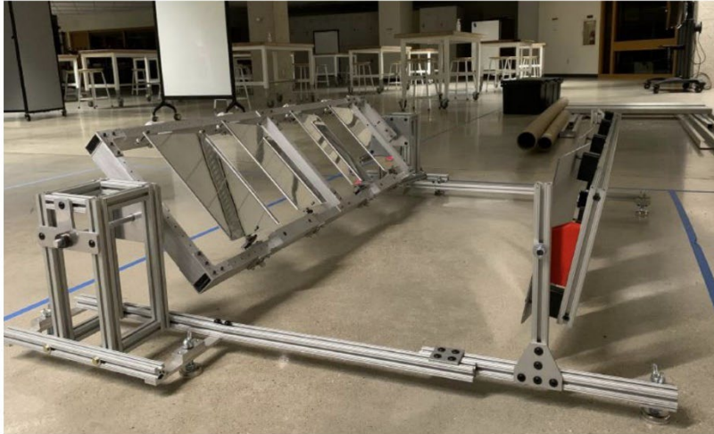
Figure 9: Prototype of the two-stage heliostat concept generated by an undergraduate senior design group. Top is an engineering model of the prototype and bottom is the completed prototype.
