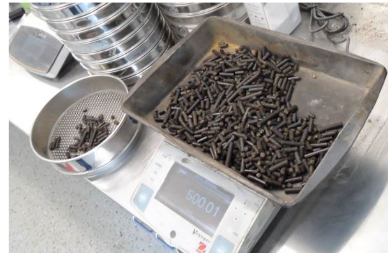
Weighing pellet sample for Pellet Durability Index test
