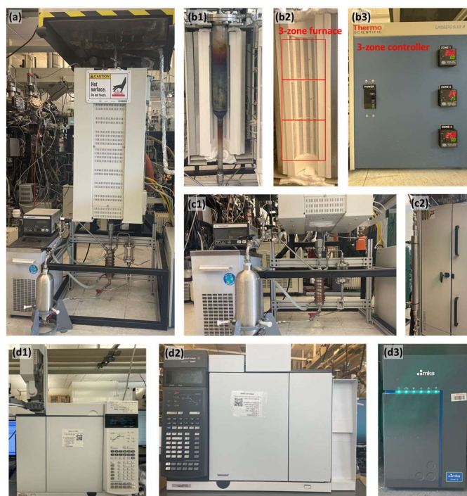
Figure 113. Photo of the current large scale reactor (a) Overall outlook (b) Reactor part with (b1) the reactor, (b2) 3-zone furnace (b3) 3-zone controller; (c) Product separation unit with the (c1) liquid condenser and (c2) the air separator; (d) Analysis part with the (d1) gas chromatography for liquid product, (d2) gas chromatography for gas product and (d3) mass spec for gas product.
