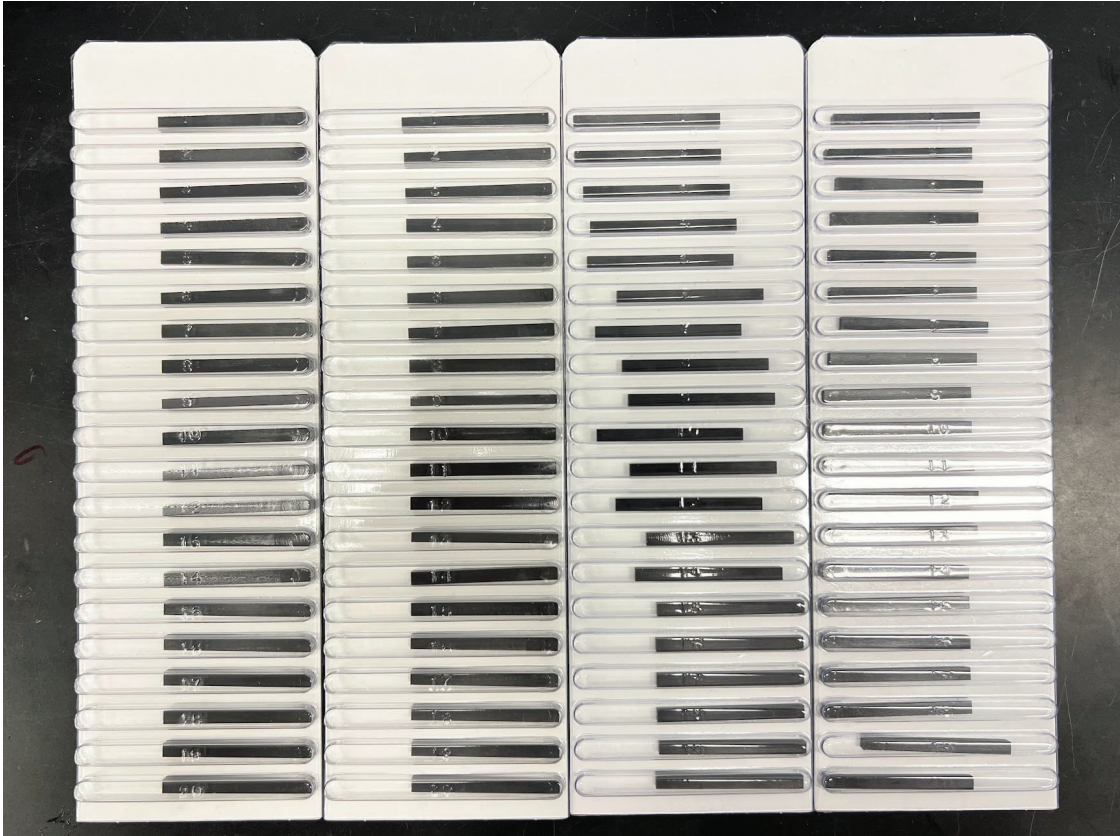
Figure 5.2: Commercial monolithic SiC samples bar samples.
