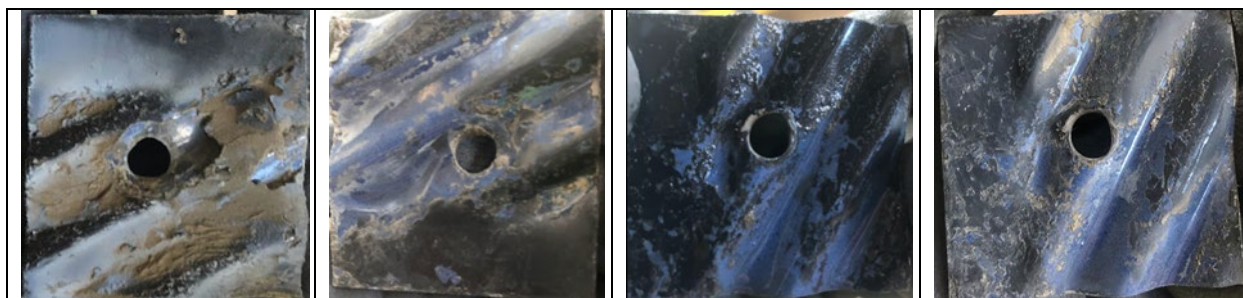
Exhibit 4.4.14. Photos of Coupon after Steps of Vacuumed, Brushed, DI Water Flushed, and Compress Air Dried Before Microscope Analysis.
