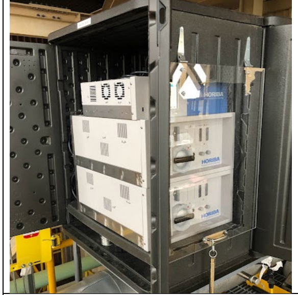
Exhibit 4.1.1. Gas Conditioner and Gas Analyzer.
