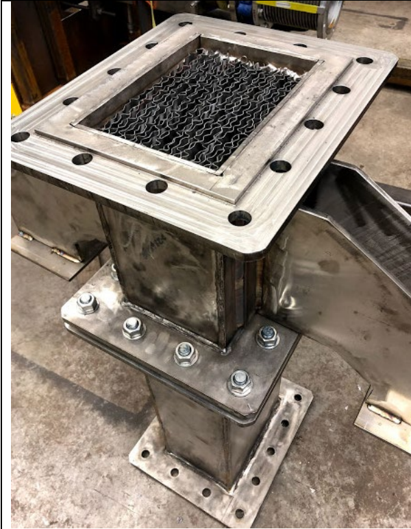
Exhibit 3.3.2 Hot End and Cold End Heating Element Sheet Packed into Housing.
