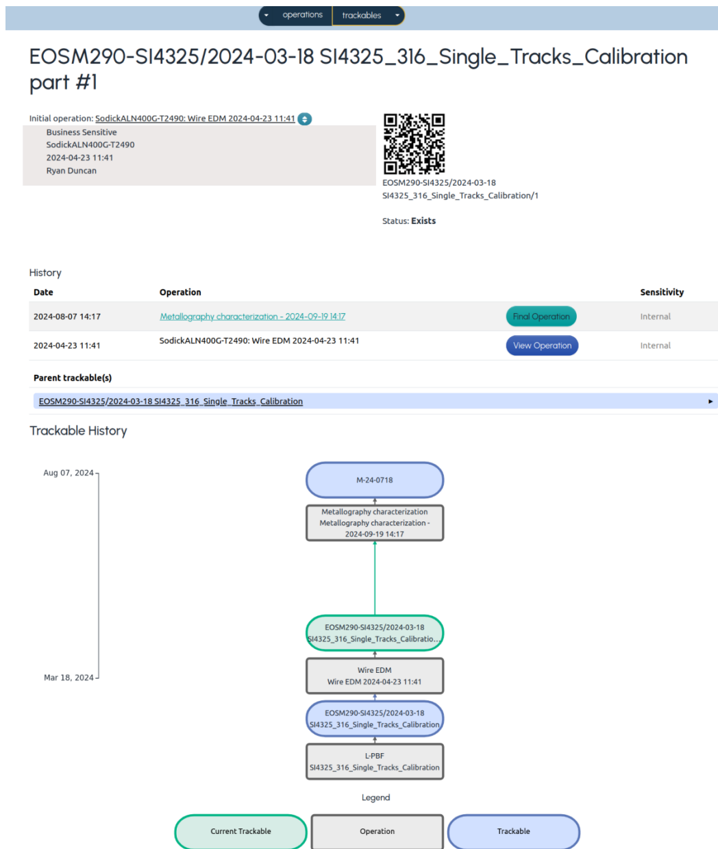
Figure 6. Trackable detail page in the Damara Tern interface. The trackable name is followed by a summary of its initial operation and basic information, including the QR code, status, and any applicable sensitivity labels. The digital thread for the trackable is presented as an expandable list of operations and parent trackables, accompanied by an interactive diagram.
