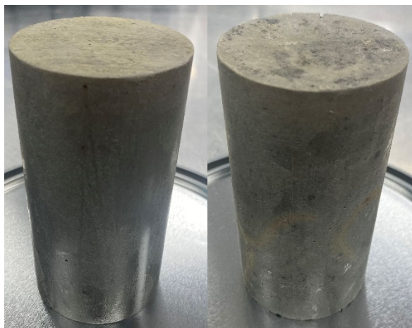
Figure 6-1. Monoliths for Cast Stone (left) and activated carbon contained Cast Stone (right)
