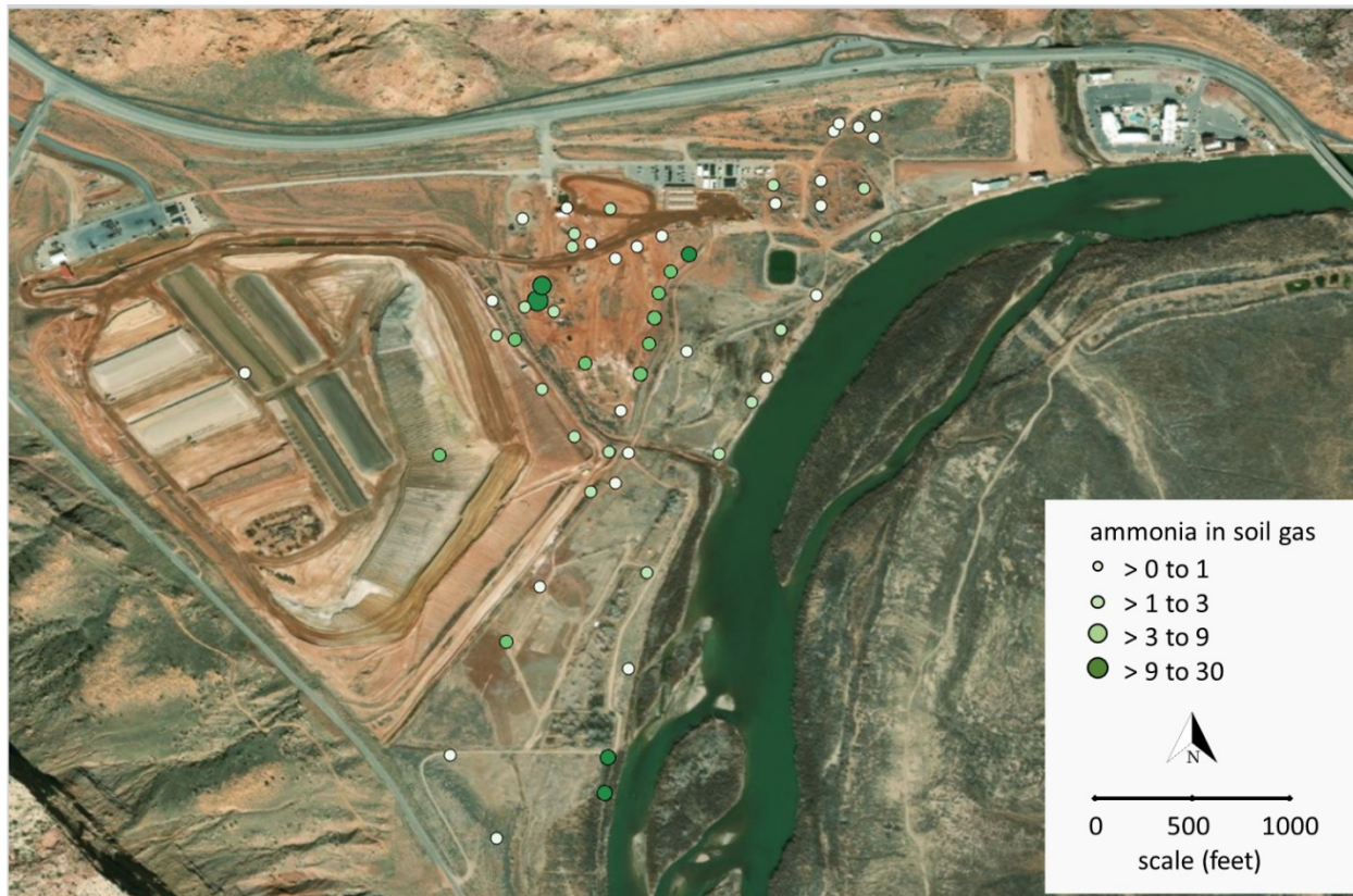
Figure 5-5. Ammonia Soil Gas Survey Data
