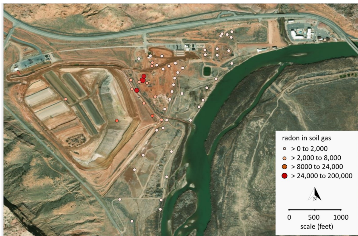
Figure 5-1. Radon Soil Gas Survey Data
