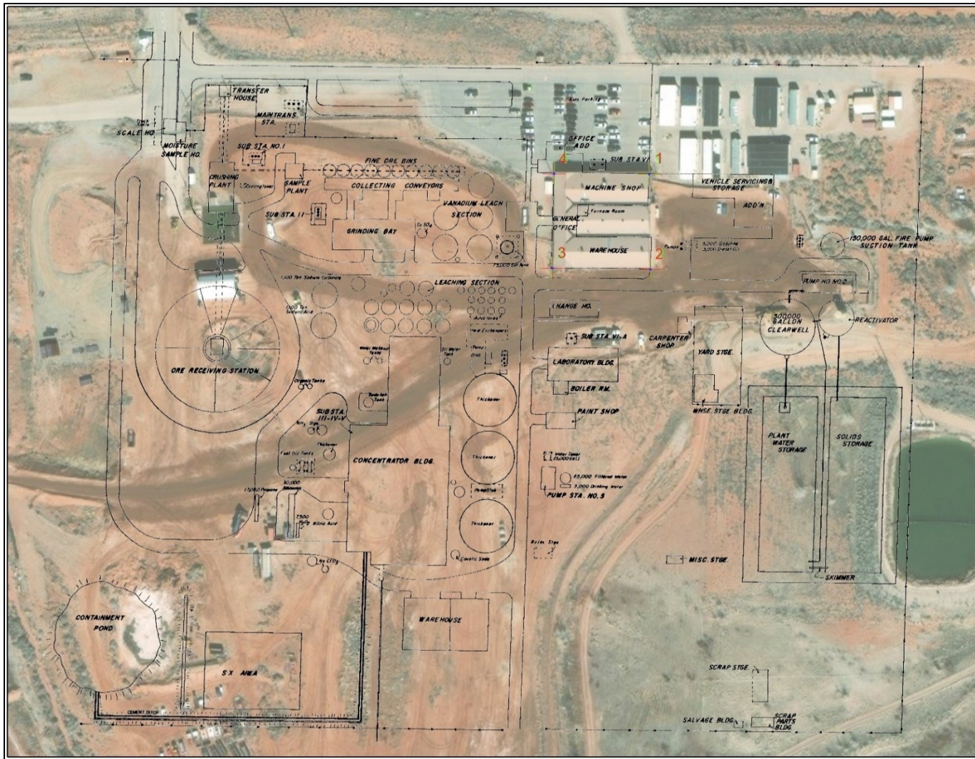
Figure 4-4. Mill Layout Diagram Overlaid Onto 2020 Satellite Imagery for Former Moab Site
