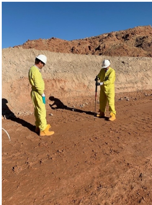
Figure 4-5. Driving a Soil Gas Probe for Soil Gas Sample Collection
