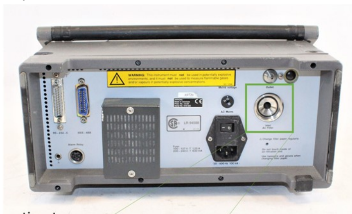
c) Connection to Tedlar bag for sample analysis
