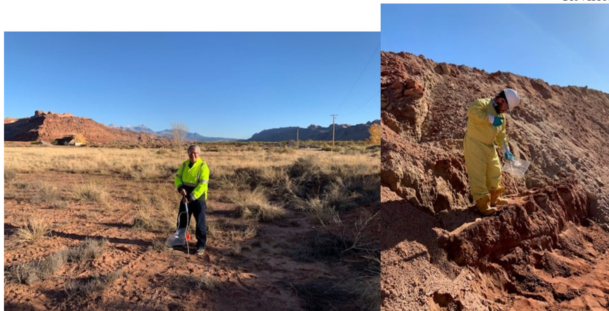
Figure 4-6. Collection of Soil Gas with Hand-Pump
