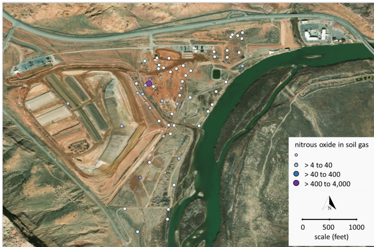
Figure 5-3. Nitrous Oxide Soil Gas Survey Data
