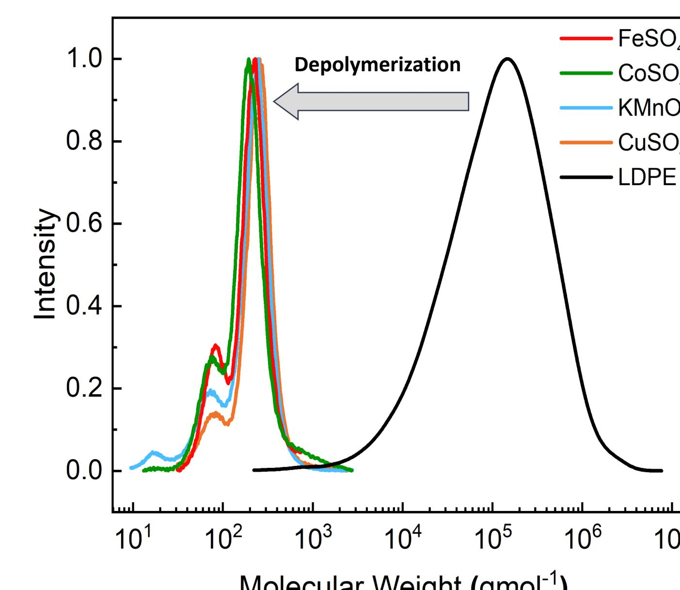
Molecular weights by size exclusion chromatography of oxidized water-soluble products (aqueous) compared to that of the original film (trichlorobenzene). The following reaction conditions were used: 10 wt % catalyst loading, 130 °C, and an initial oxygen pressure of 7 bar.
