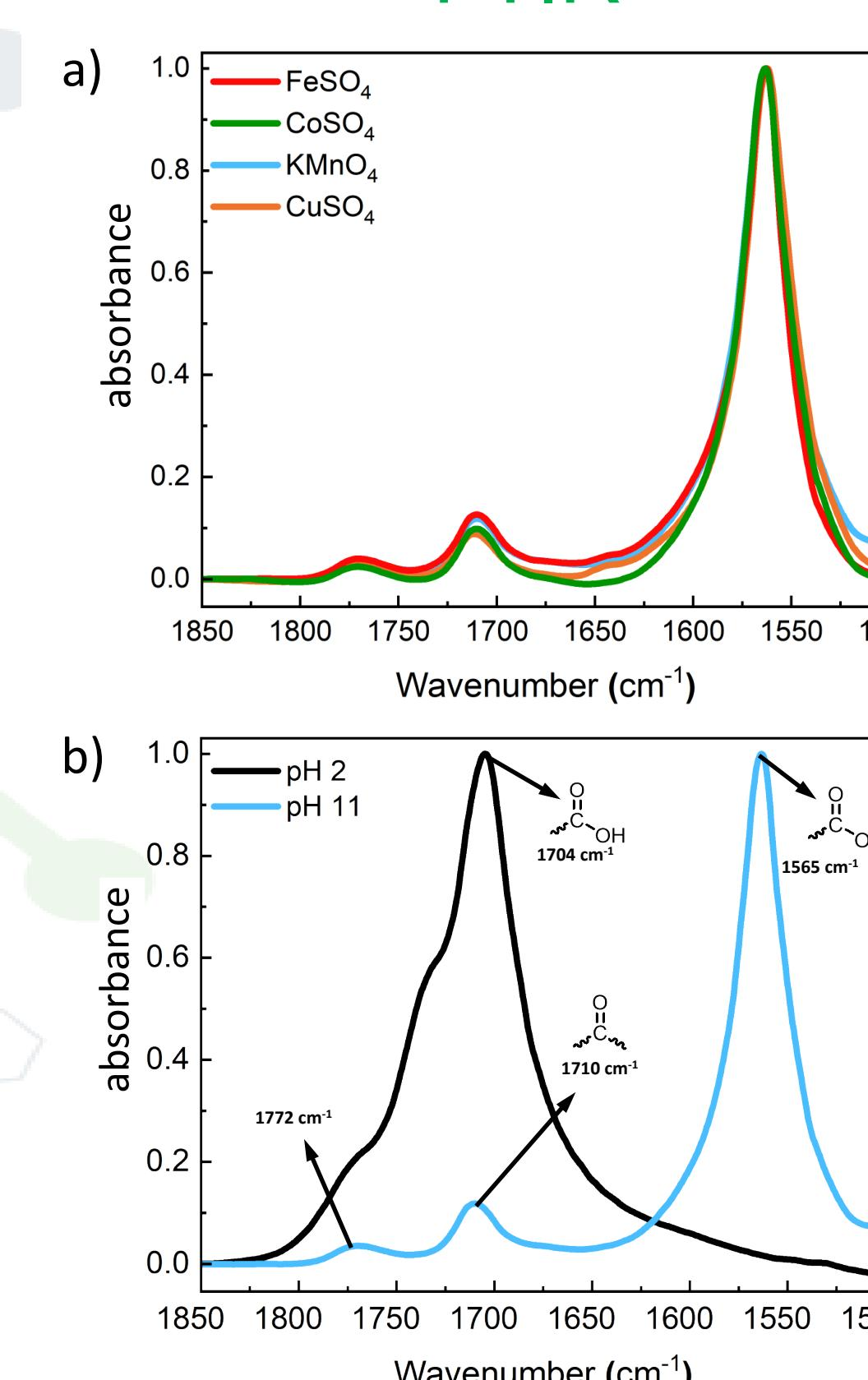
a) Representative FTIR spectra for the water-soluble oxidized products at pH 11. Reactions were run using 10 wt % catalyst, 130 °C, and an initial oxygen pressure of 7 bar. b) FTIR spectra for the water-soluble oxidized products of the reaction with KMnO<sub>4</sub> at pH 2 and pH 11.
