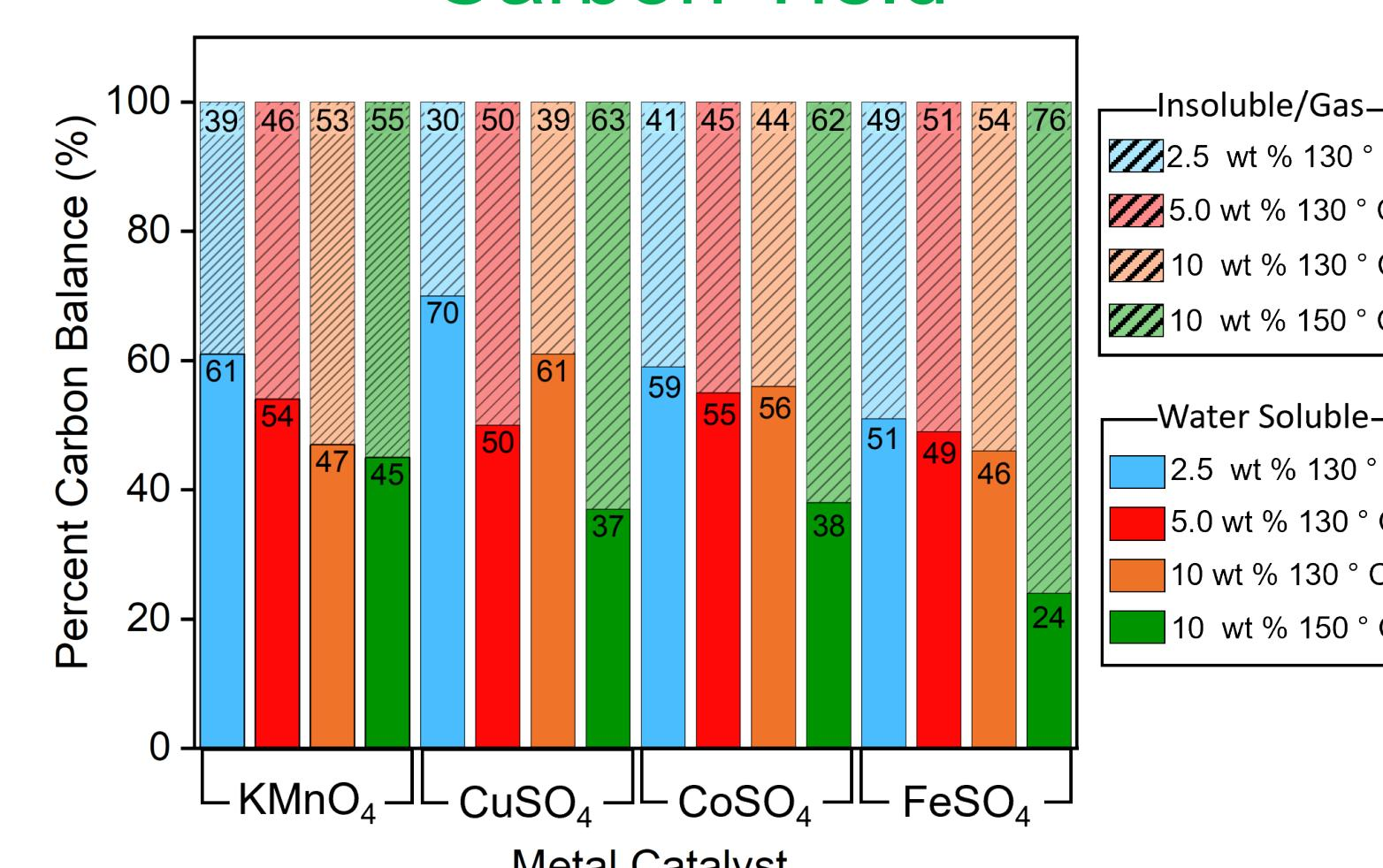
Carbon balance after LDPE oxidation using various catalyst concentrations and reaction temperatures. Using elemental analysis, percent carbon was determined by comparing carbon recovered in the water-soluble products with the carbon content of the initial LDPE film. The percent carbon present in insoluble material or volatile compounds was determined as the difference between the carbon of the initial LDPE film and that recovered in water soluble products.
