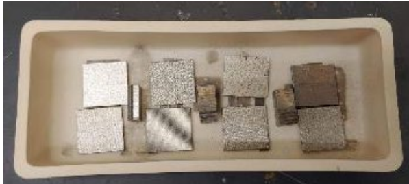
Images of the samples in crucible for the heat treatment
