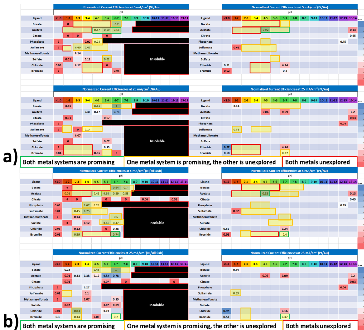
Figure 55. Heat maps of normalized current efficiency for a) First-pass Ni and Pt depositions and b) Second-pass Ni and Pt depositions. Ni depositions are on the left, Pt on the right. 5 mA/cm 2 was used for the top maps while 25 mA/cm 2 was used for the bottom maps. Chemistry/ligands are displayed in the row headers while pH ranges are displayed in the column headers. Each cell represents the average normalized current efficiency measured for the given experimental conditions.
