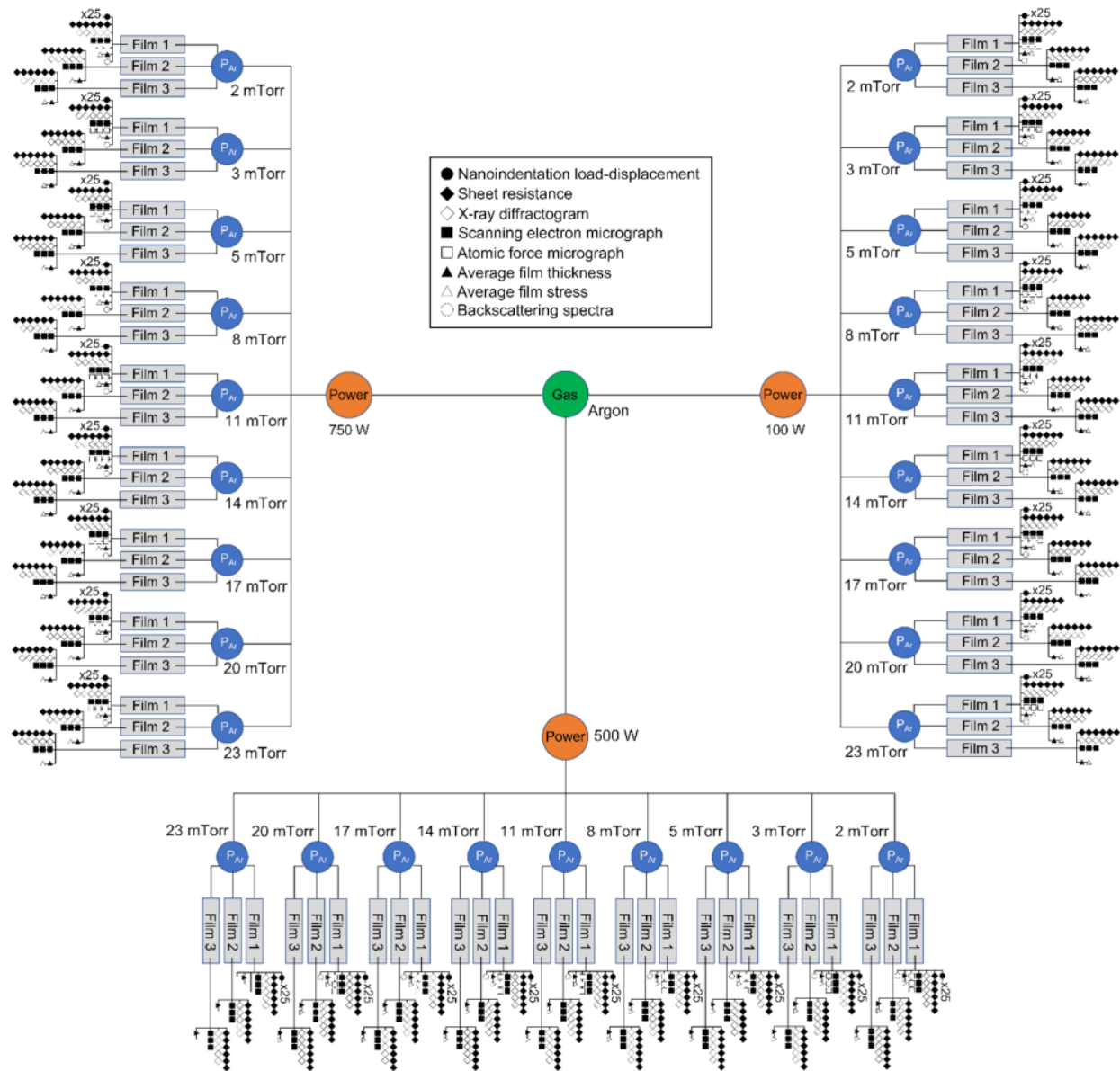
Figure 15. A summary of the 2,072 measurements performed on a combinatorial library of pure Mo films deposited under a range of conditions and characterized via several complementary modalities.
