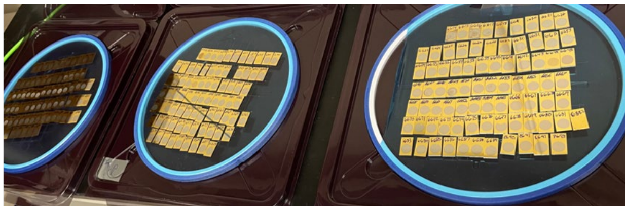
Figure 54. 200 Ni plated samples plated using the high throughput tooling over the course of one afternoon.
