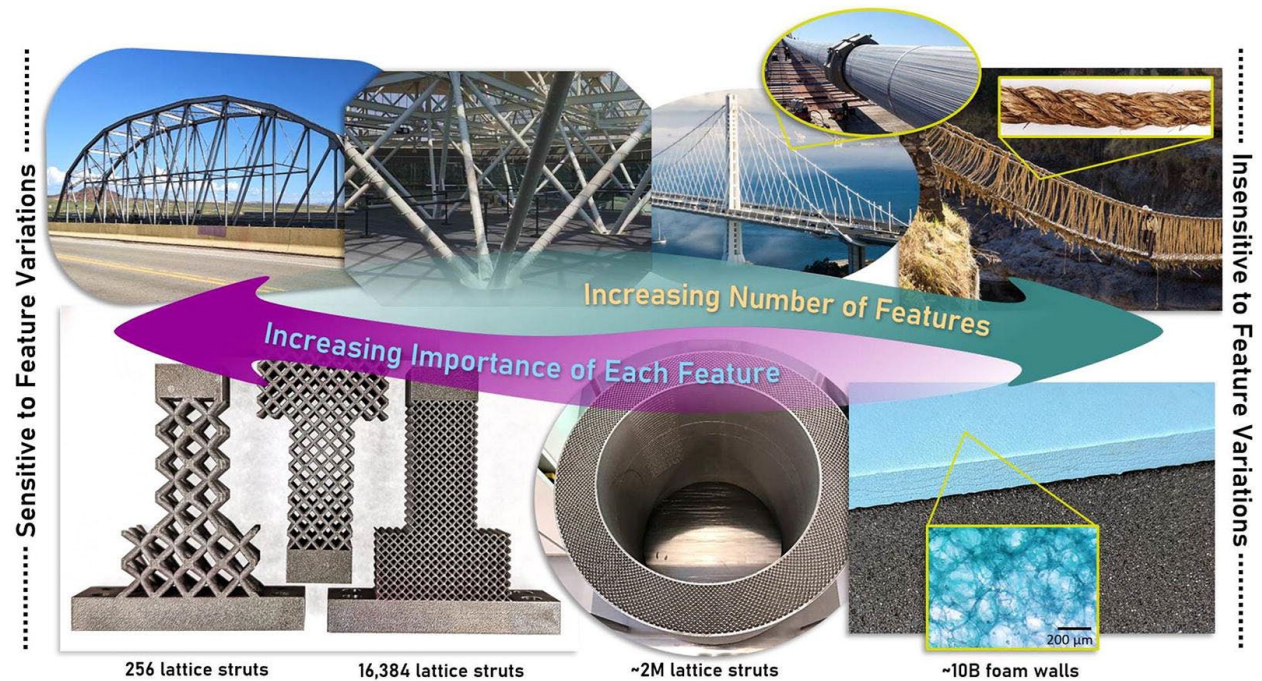
Figure 2. High-throughput testing allows rapid assessment of stochastic material variability. Here, applied to additively manufactured lattices, high-throughput testing reveals that the effective variability in material stiffness decreases as the number of unit cells increase due to a homogenization effect.
