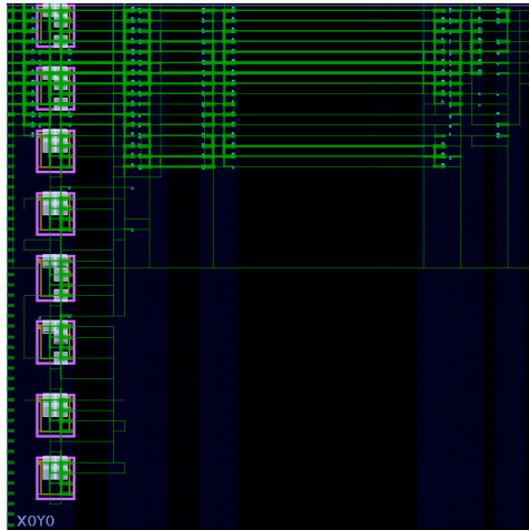
Figure 2.3: Vivado implementation view showing layout of the SR-PUF hard macros.
