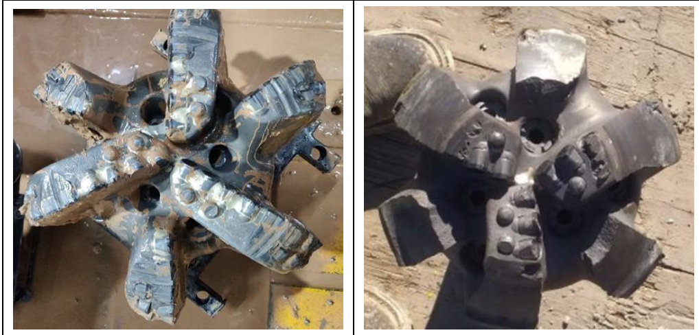
Figure 6-4. Damage beyond repair caused by blade shear: a) Bit 5 on 16A(78)-32, b) Bit 19 on 16A(78)-32.
