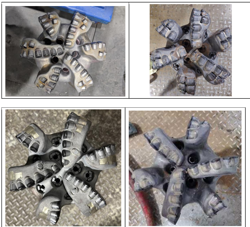
Figure 6-3. Normal wear and test observed on representative bits: a) NOV Bit 26 on 16A(78)-32 drilled 742 ft @ 42 ft/hr, b) Smith Bit 8 on 16A(78)-32 drilled 232 ft @ 13 ft/hr, c) Baker Hughes Bit 19 on 16B(78)-32 drilled 670 ft @ 78 ft/hr, and d) Ulterra Bit 9 on 16A(78)-32 drilled 124 ft @ 14 ft/hr.
