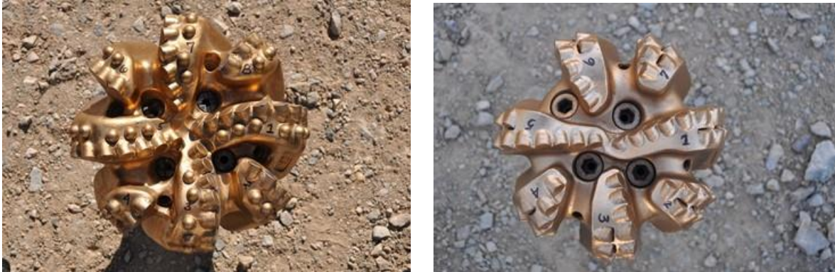
Figure 2-2. Drag Bit Design Feature Description. Eight blade bit (left) with Torque Control Components and Impact arrestors and Seven Blade bit (right) with Backup cutters (Ref: Raymond et al, GRC 2012.)
