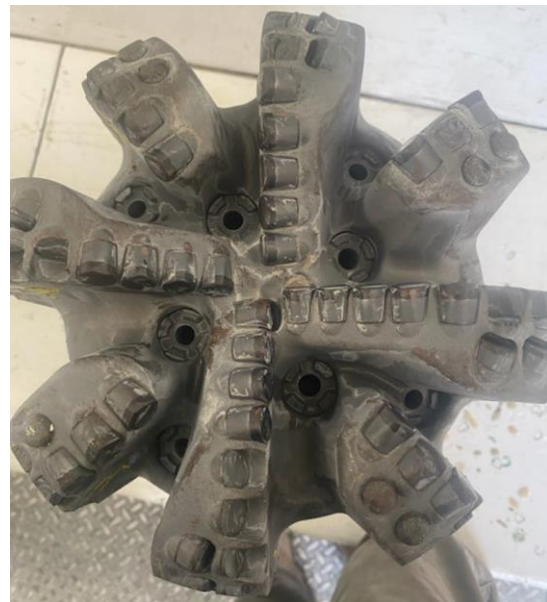
Figure 3-7. Post-drill photo of bit #13.
