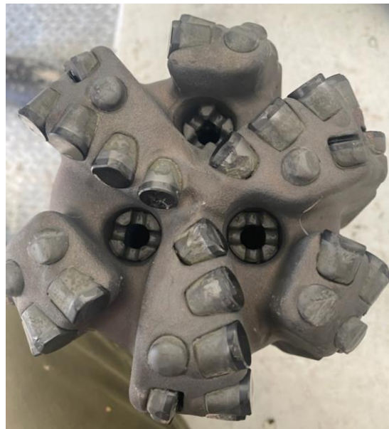
Figure 3-9. Post drill photo of bit #17.
