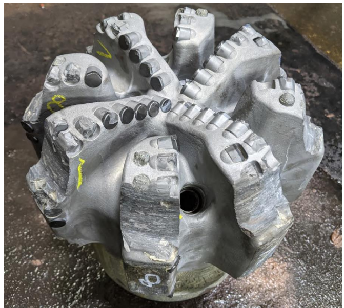
Figure 3-4. Post-Drill Photo of Bit #7.
