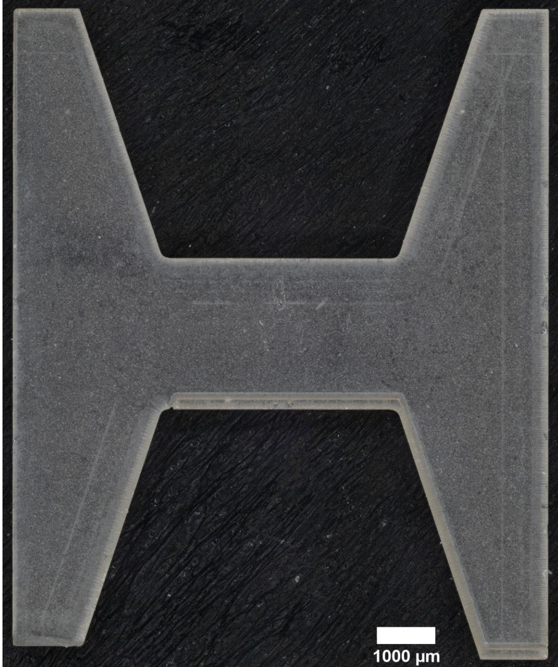
Figure 4: A bowtie shape cut out of a 6" C-Plane sapphire wafer to demonstrate the capability of fabricating non-rectangular ion traps from a sapphire substrate. Multiple passes and adjustments were needed to singulate this shape, which can be seen in the additional dicing mark near the bottom of the isthmus.
