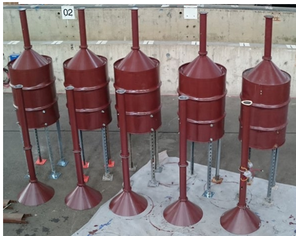
Figure 2. Assembled array of five oscillating water columns (OWCs)
