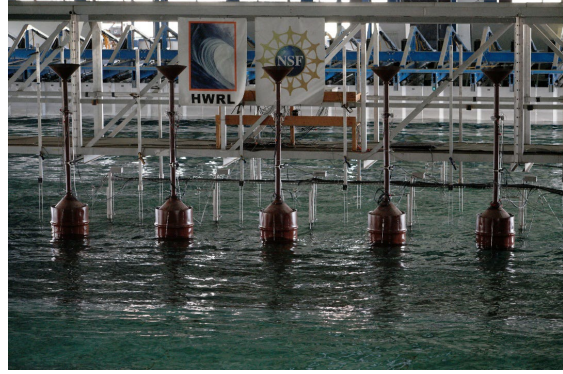
Figure 7. Nonoptimized (l) and optimal (r) OWC array layouts in tank testing
