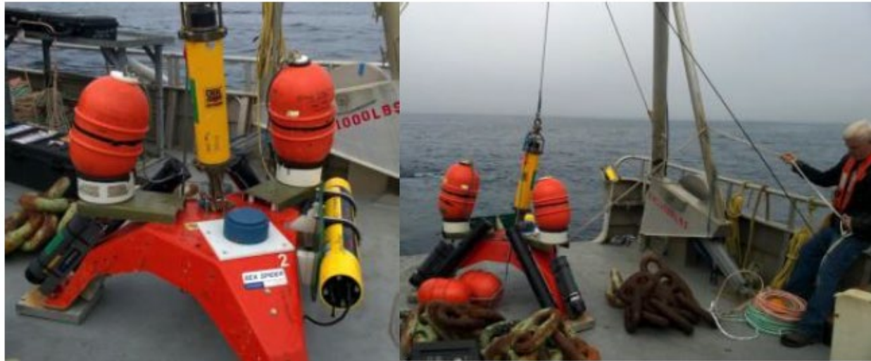
Figure 3. Preparation (left panel) and deployment (right panel) of SeaSpider acoustic package at PacWave South Energy Test Site (SETS), April 2016.
