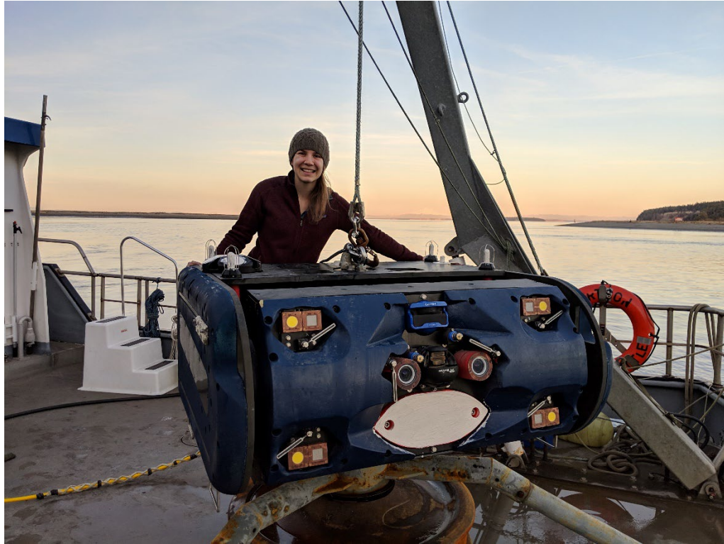
Figure 4. The 3G-AMP prior to deployment in Sequim Bay. The sensor package includes stereo-optical cameras, an echosounder, two imaging sonars, an ADCP, and a hydrophone array. Biofouling mitigation (mechanical wipers and UV lighting) are integrated with most sensors and the pitch angle of the sensors can be adjusted by an internal motor.
