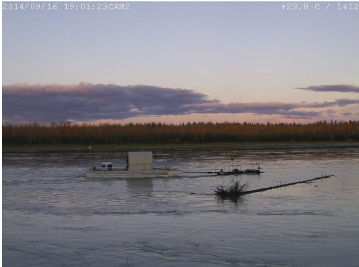
Figure 6. Test barge with an Oceana Energy, Inc. turbine on deck behind the instrument tent, tethered behind the RDDP at the Tanana River Test Site, Alaska. A large debris object floats downstream nearby. (Photo from the Video Debris Observation System)
