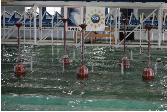
Figure 7. Nonoptimized (l) and optimal (r) OWC array layouts in tank testing
