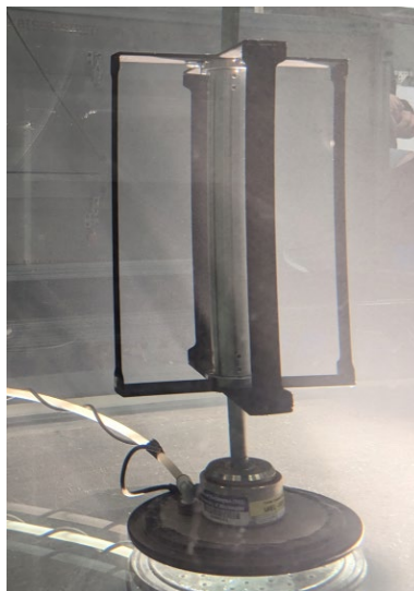
Figure 43: Scale-model turbine in the Tyler Flume. The blade-strut connection (blade ends) deviates from the actual turbine (Figure 11) due to the size of the mounting hardware required.
