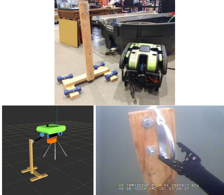
Figure 12. Photograph, onboard camera still image and ROS rviz visualization (clockwise from top left) of grasp target for shallow-water intervention trial (note that the time and date on the video overlay are incorrect, the trial was conducted on 19 June 2017).
