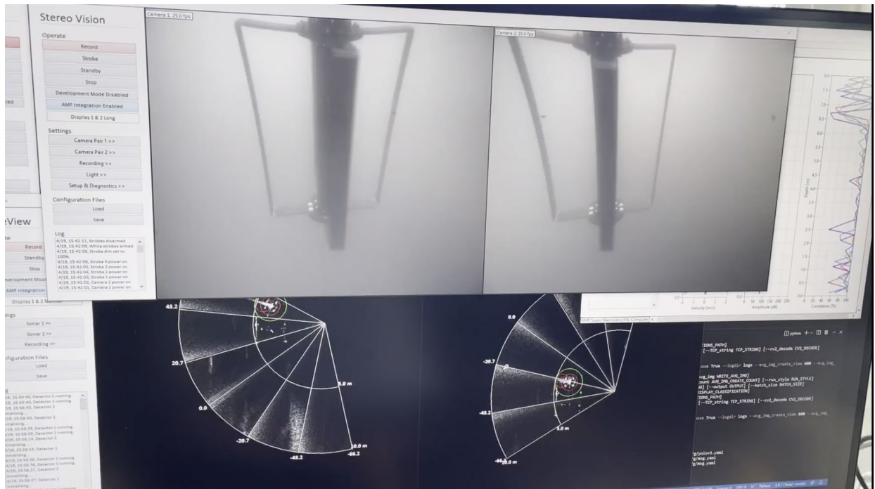
Figure 10: Optical and sonar images of the turbine during deployment. This display was visible aboard the vessel and used to populate a log of events of interest by the real-time observer.
