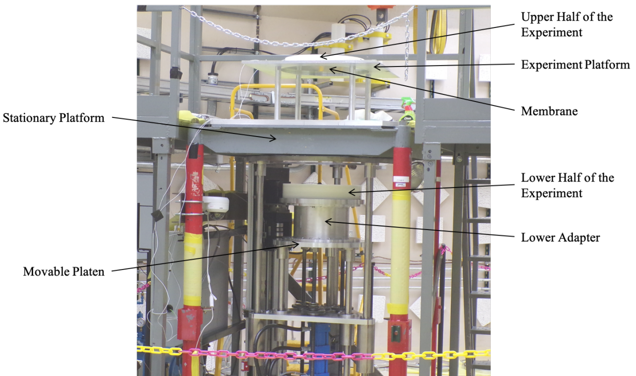
Figure 3: The Comet general purpose critical assembly machine. The Godiva IV fast burst reactor is located to the right of this photo (out of frame).
