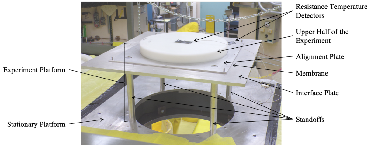
Figure 4: Upper stationary platform of the Comet, with the experiment platform. During the benchmark measurements, the resistance temperature detectors and alignment plate were removed.
