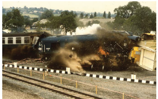
Fig. 5. CEGB public demonstration test with the Magnox spent fuel flask. [22] © Nuclear Decommissioning Authority.
