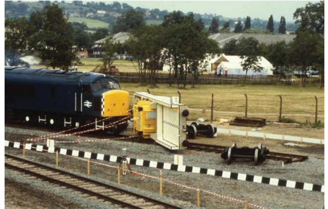
Fig. 4. Configuration of the full-scale crash test of the Magnox spent fuel flask. [22] © Nuclear Decommissioning Authority.
