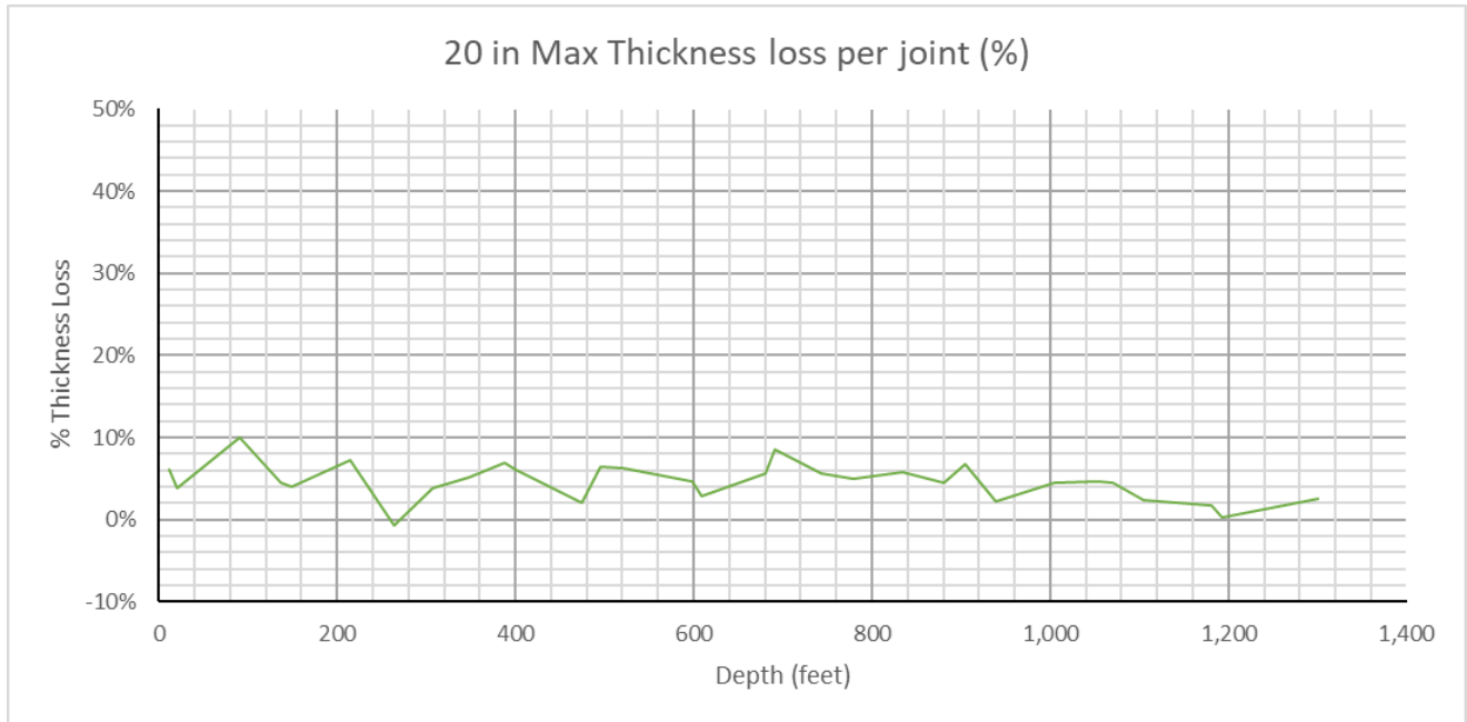
Figure 4-5. BM-111B pipe thickness loss for the 20" casing
