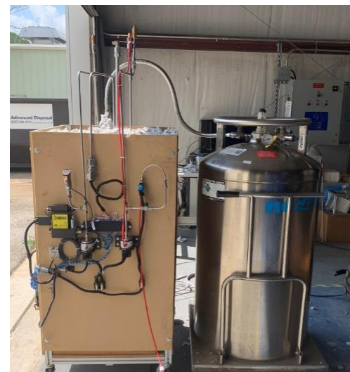
FIGURE 2. TEST VESSEL WITH LIQUID NITROGEN CONNECTED TO COOLING CHANNELS
