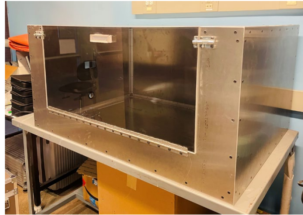
Figure 9. High voltage test enclosure for multi-kV isolation testing of planar transformers in this project. The 0.09" aluminum enclosure is 5' x 3' x 2' and is solidly connected to earth. The viewing window is 0.25" Lexan.
