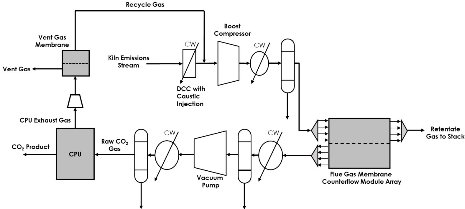
Note: CW = cooling water; DCC = direct contact cooler; CPU = compression and purification unit
