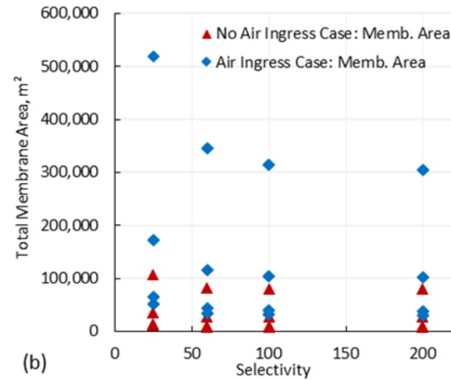
The reduction in the volumetric flow of the treated emission stream contributes to a reduced system size, capital cost, energy usage, and O&M cost. Moreover, increasing the membrane CO<sub>2</sub> selectivity reduces the total membrane area.
