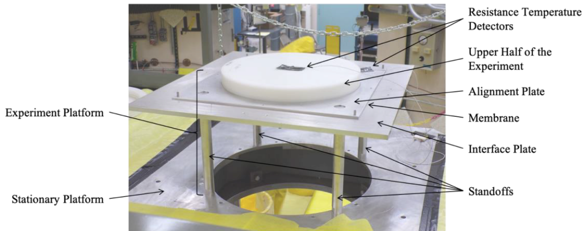
Figure 5: Upper stationary platform of Comet, with the experiment platform.
