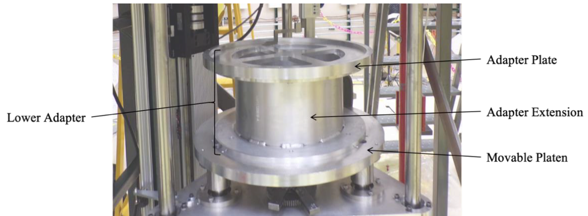
Figure 6: Lower movable platen of Comet, with the lower adapter from TEX-Hf.
