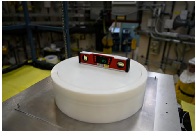
Figure 23: Levelness measurements being performed for the top stack.
