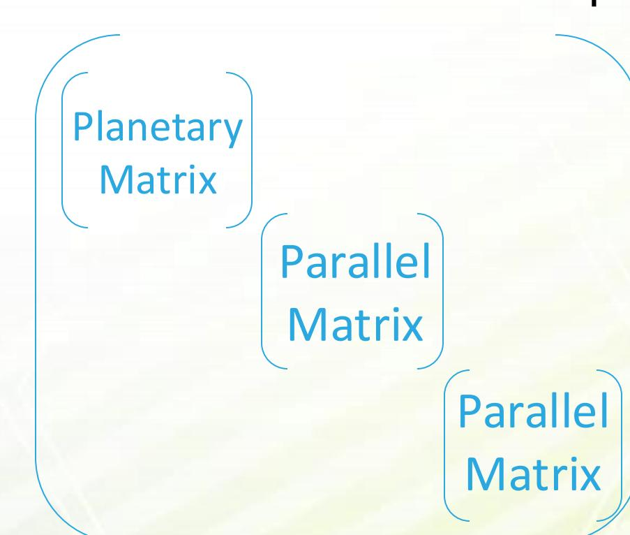
Fig. 5: Depiction of a lump-parameter matrix configured to represent a planetary-parallel-parallel gearbox. The matrix is 10x10, and the matrices are overlaid with their diagonals along the main diagonal. All elements that are not representing a gear stage component are zeros. The stiffness and inertia matrices are configured in this way, while the state vectors are simply vertically concatenated.
