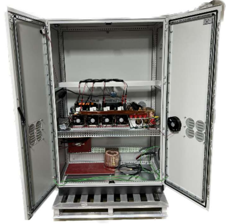
Fig. 8. Image of 1 kV class 150 A isolated DC/DC converter based on DAB.
