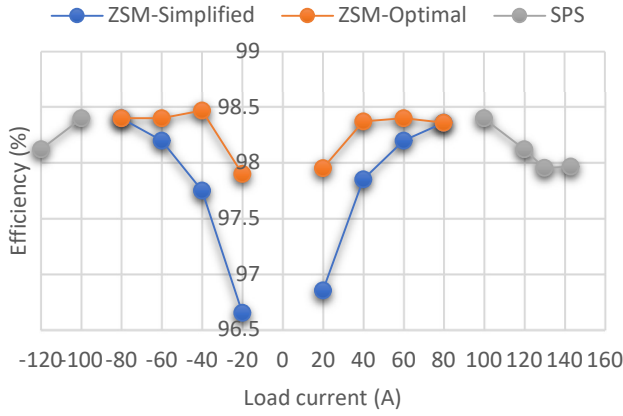
Fig. 16. Measured efficiency at 900 V for different operating modes.
