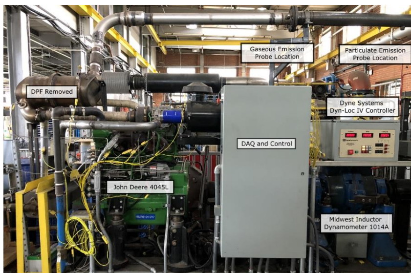
Figure 6.1. Image of the John Deere 4045L test engine and the associated data acquisition and control systems.
