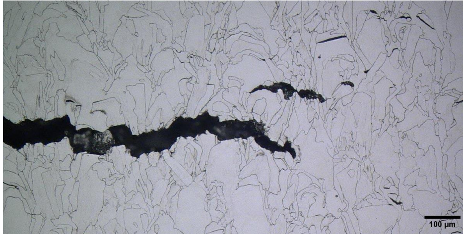
Figure 5.10. Cross section of crack in SA specimen LCF-6, creep-fatigue tested at 550 °C with a \Delta\epsilon of 1% and a hold time of 6 minutes.
