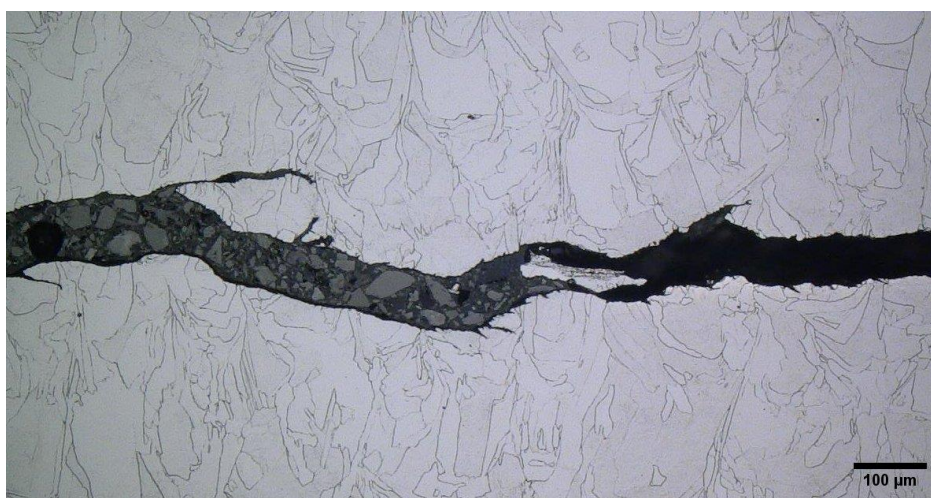
Figure 5.6. Cross section of crack in SA specimen LCF-7, fatigue tested at 550 °C with a \Delta\epsilon of 1%.
