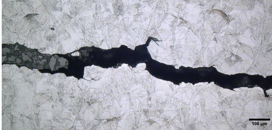
Figure 5.7. Cross section of crack in SR specimen LCF-4, fatigue tested at 650 °C with a \Delta\epsilon of 1%.
