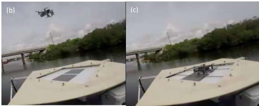
Fig. 10. Flight Deck: (a) Full view of the flight deck onboard the WAM-V16 platform; (b) View of the flight deck before drone landing; (c) View following the drone landing
