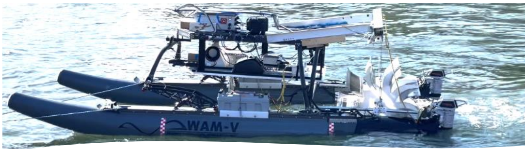
Fig. 1. The completed MHK Platform in operation in tidal waters of the Intracoastal Waterway in South Florida
