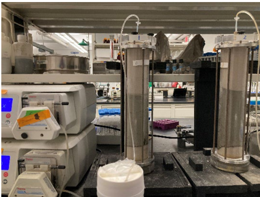
Figure 3-1 Setup of column leaching test
