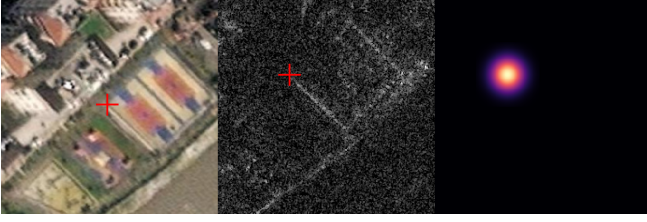
Fig. 2. A SAR keypoint detection training sample. An optical (left) and SAR (center) image is cropped centered at the location of the optical keypoint and a heatmap label (right) is created with a Gaussian located at the SAR keypoint location. Optical and SAR keypoint locations are indicated in red.
