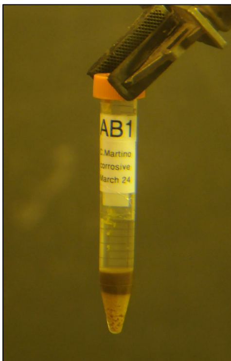
Figure 3-4. Sequentially pH Adjusted ABD Material and Depleted Uranium Material, After Settling.
