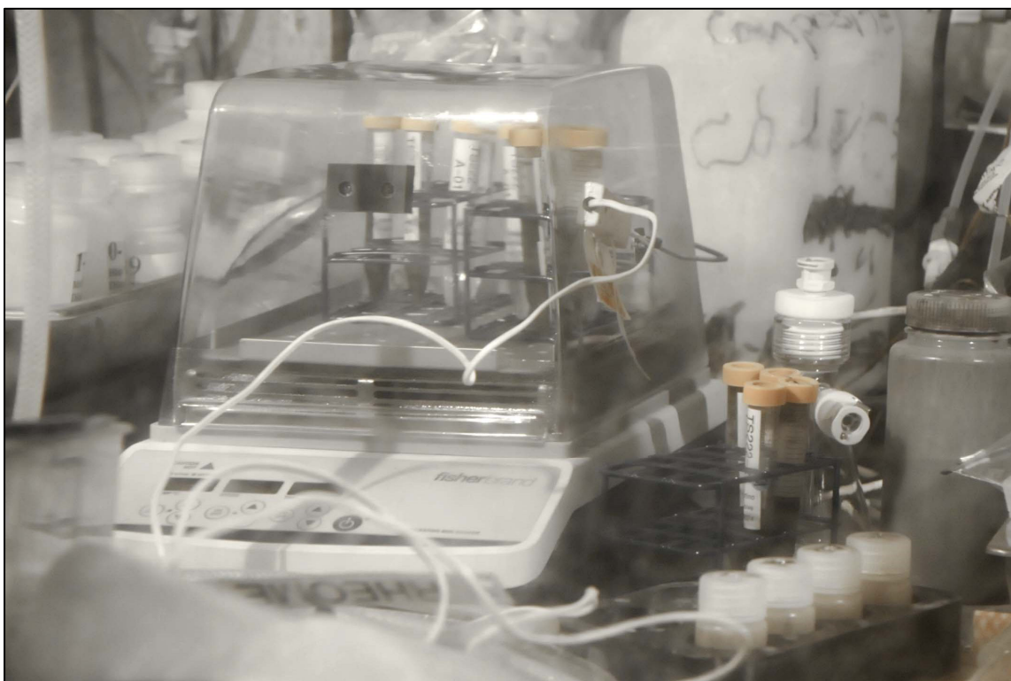
Figure 2-4. Heated Shaker Table Used in Cell 2.
