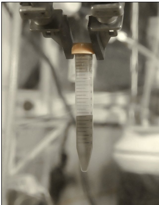
Figure 3-5. Settled Mixture of ABD Material and CSTF Sludge at Completion of a Series C Test.
