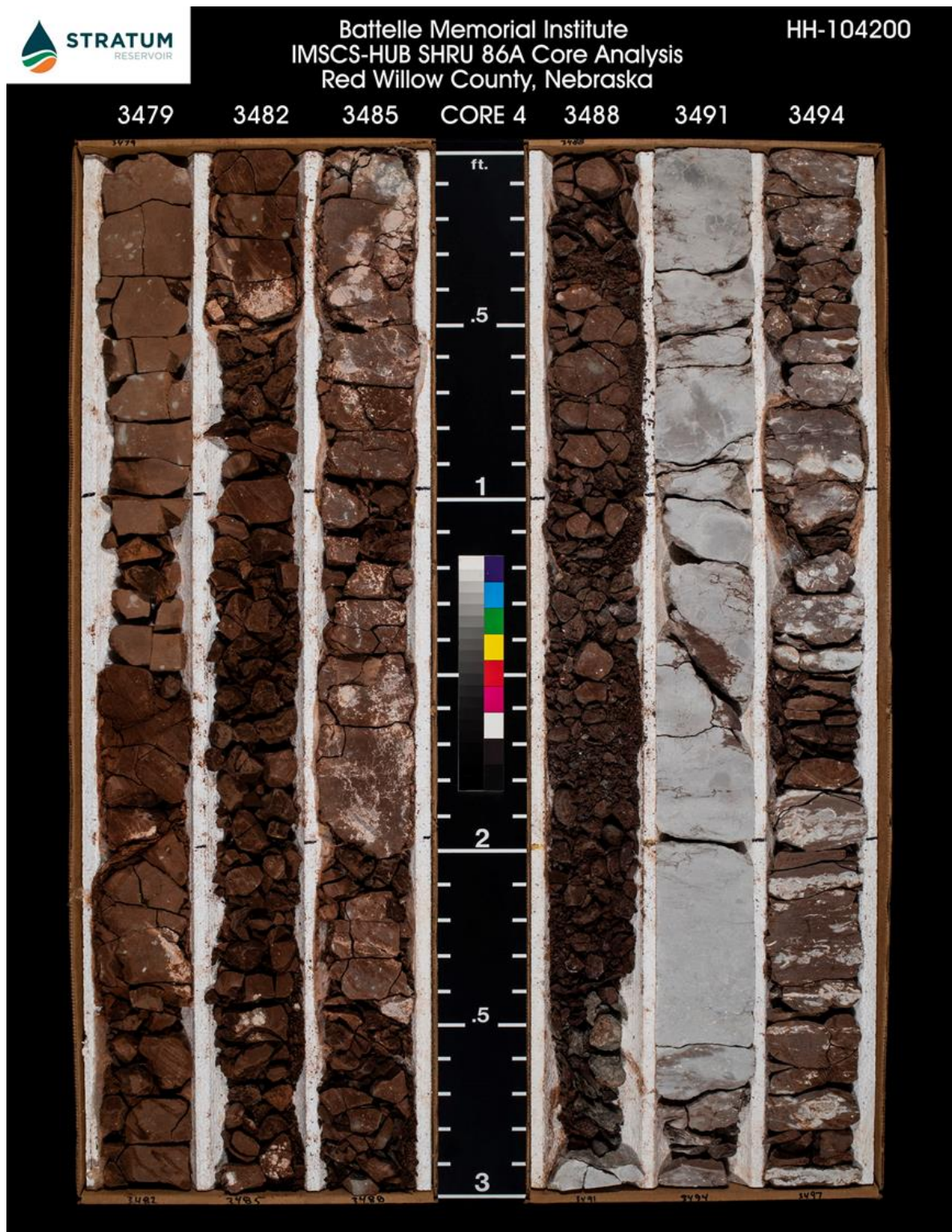
Figure 8: Core 4 from the IMSCS-HUB SHRU 86A well, depth 3,479-3,497 ft. Scale (middle) is in feet and tenths of feet.
