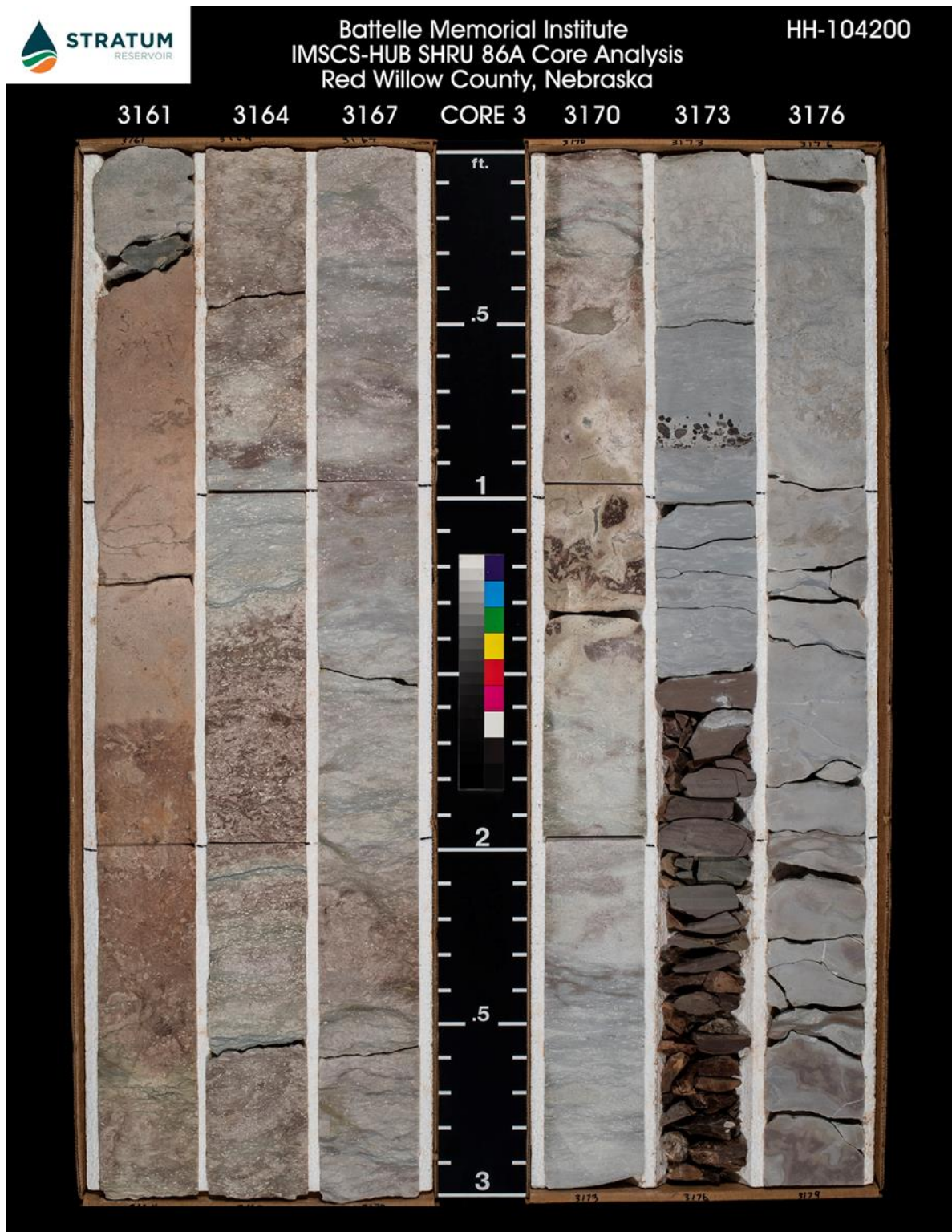
Figure 6: Core 3 from the IMSCS-HUB SHRU 86A well, depth 3,161-3,179 ft. Scale (middle) is in feet and tenths of feet.
