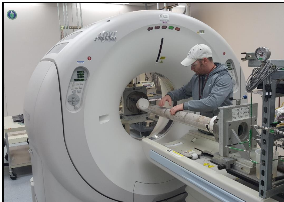
Figure 12: Toshiba® Aquilion™ TSX-101A/R medical scanner at NETL used for core analysis.
