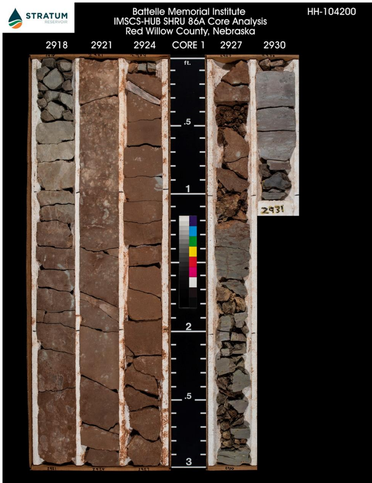
Figure 3: Core 1 from the IMSCS-HUB SHRU 86A well, depth 2,918-2,931 ft. Scale (middle) is in feet and tenths of feet.
