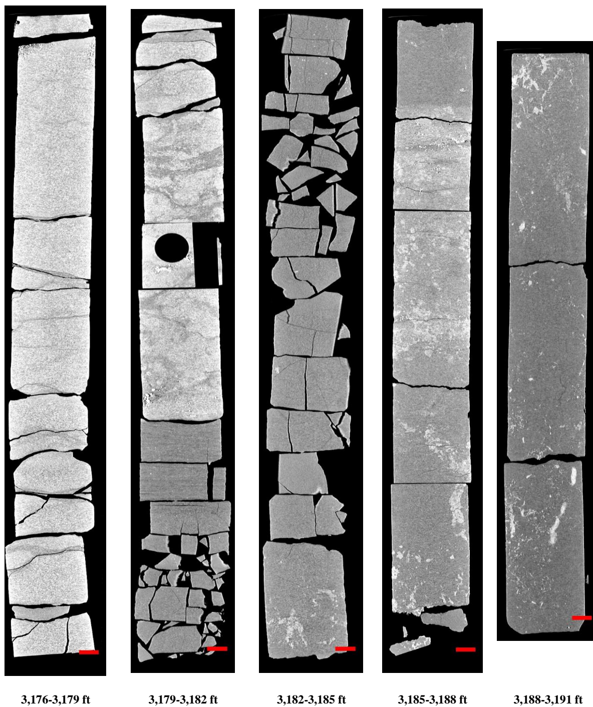
Figure 23: 2D isolated planes through the vertical center of the medical CT scans of the IMSCS-HUB SHRU 86A well Core 3 from 3,176 to 3,191 ft.
