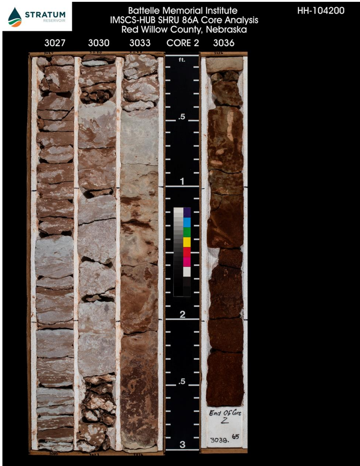
Figure 5: Core 2 from the IMSCS-HUB SHRU 86A well, depth 3,027-3,038.65 ft. Scale (middle) is in feet and tenths of feet.
