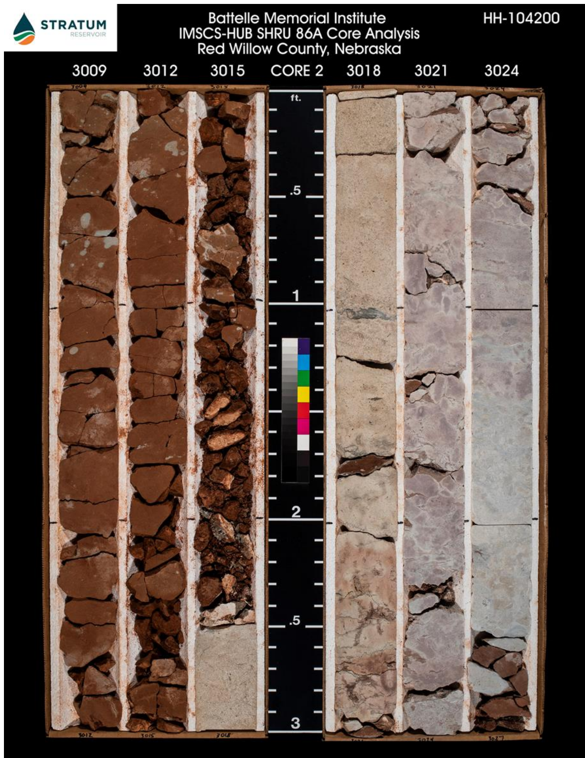
Figure 4: Core 2 from the IMSCS-HUB SHRU 86A well, depth 3,009-3,027 ft. Scale (middle) is in feet and tenths of feet.
