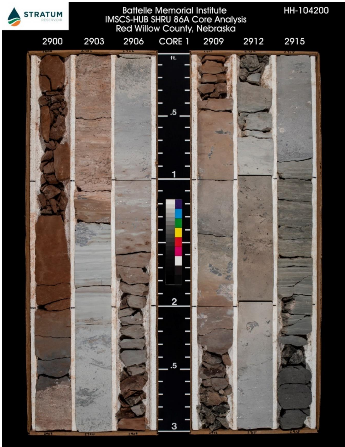
Figure 2: Core 1 from the IMSCS-HUB SHRU 86A well, depth 2,900-2,918 ft. Scale (middle) is in feet and tenths of feet.
