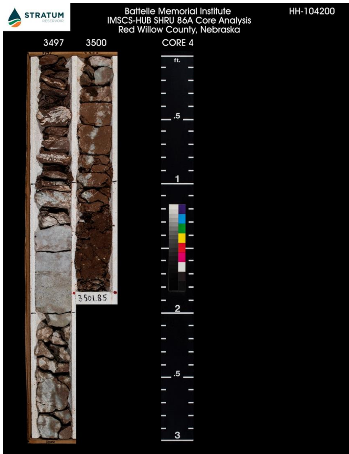
Figure 9: Core 4 from the IMSCS-HUB SHRU 86A well, depth 3,497-3,501.85 ft. Scale (middle) is in feet and tenths of feet.
